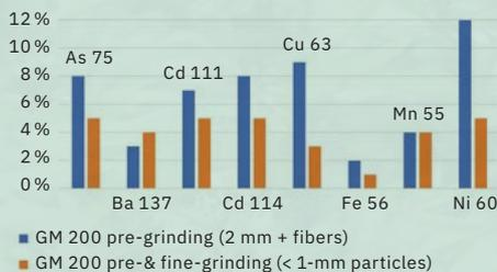
Figure 11: Particle size effects on the reproducibility of heavy metal analysis in cannabis flowers. After 10 s of grinding (interval at 4,000 rpm) in the GM 200 knife mill, fibers remain; the corresponding standard deviations in the heavy metal analysis are higher than for samples ground for 20 s with final finenesses of < 1 mm (10-s interval, 4,000 rpm + 10 s at 10,000 rpm).
