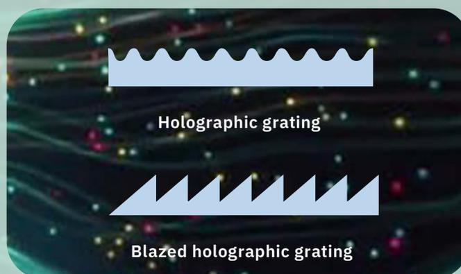
Figure 3: Groove shape of diffraction grating
