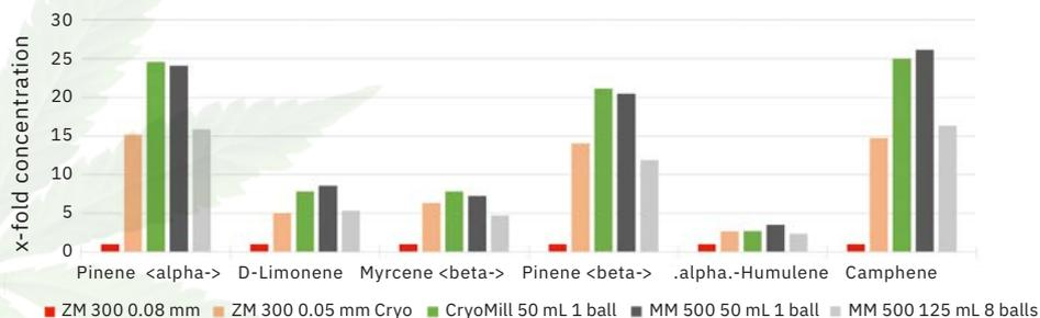
Figure 6: If the sample gets too warm (provoked in the ZM 300 with a 0.08-mm sieve), the terpenes evaporate. If a sieve with larger apertures is selected and the sample is processed cryogenically, loss of the volatile components can be minimized. The best results are achieved in closed ball mills (CryoMill, MM 500 control) with cryogenic grinding.
