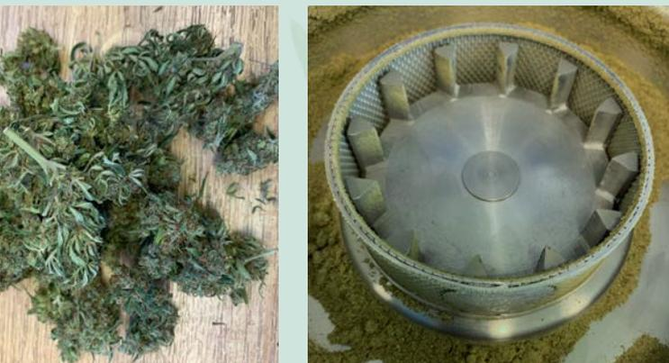
Figure 8: Cannabis flowers before grinding and after cryogenic grinding in a ball mill (total of 4 min for 20 g sample) or the ZM 300 (10 min for 500 g sample)
