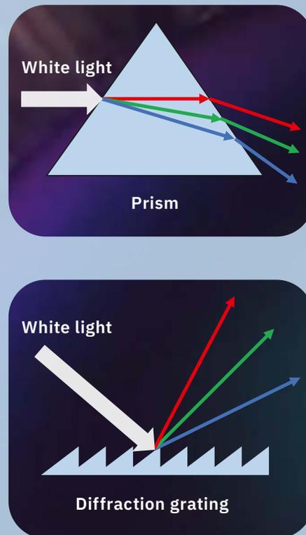
Figure 2: Principles of prism and diffraction grating
