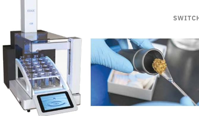
Figure 3: The EDGE from CEM (left). Filling the homogenized sample into the Q-Cup before extraction (right).
