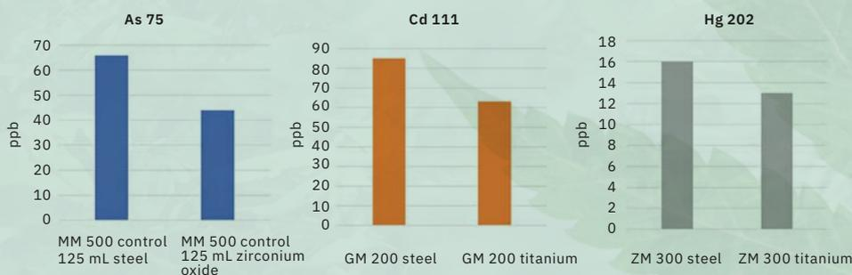
Figure 12: Effects of the correct grinding tool on analysis results. The abrasion from steel tools leads to higher heavy metal values, which distorts the analysis. This can be avoided by using zirconium oxide or titanium tools.
