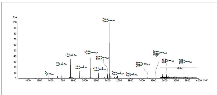
MALDI MS Spectrum of 2-AA labeled N-glycan prepared from a human plasma sample. The peak profile can be directly converted to and interpreted as the glycan expression profile.
