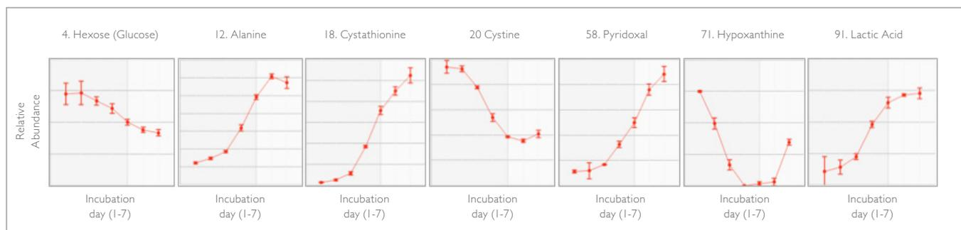
Representative results of a time-course experiment demonstrate consumption and accumulation of critical media components.
