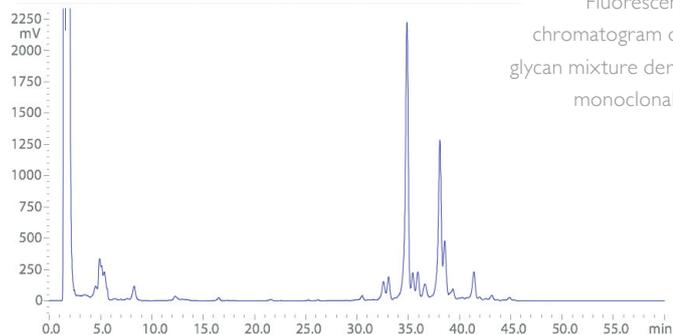
Fluorescence HPLC chromatogram of labelled glycan mixture derived from monoclonal antibody sample.
