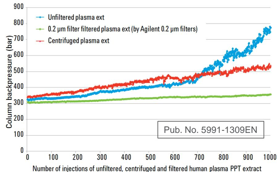
Unfiltered, centrifuged, and filtered plasma extracts
