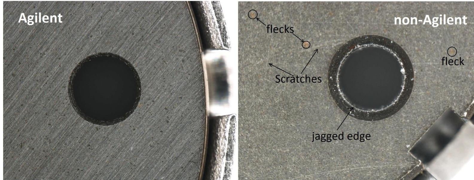
*Photomicrographs of rotor seal from Agilent and other vendor*
