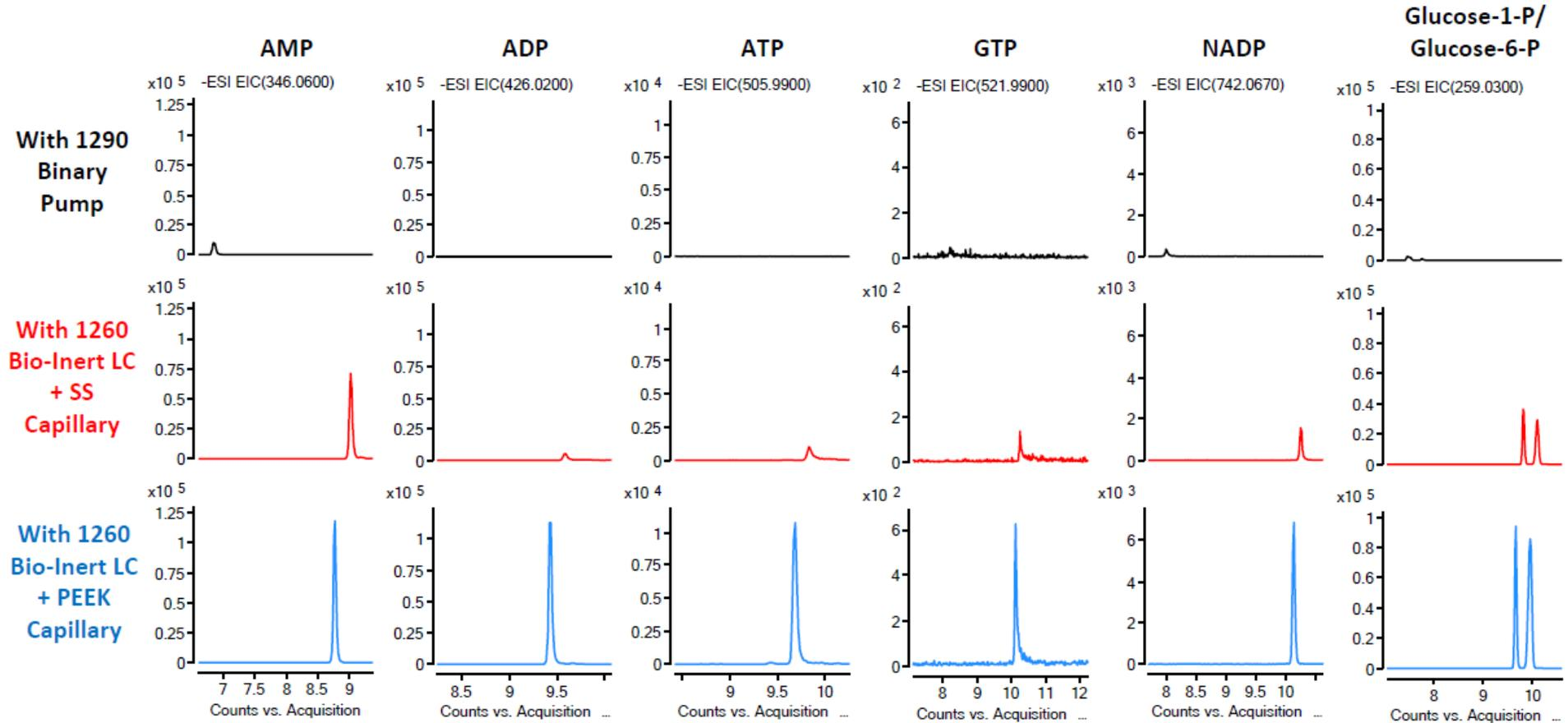
Column used was 2.1 x 100 mm, 2.7  $\mu$ m Agilent InfinityLab Poroshell 120 HILIC-Z (PEEK lined stainless steel); A: 10 mM Ammonium Formate pH 6.8 in water, B: acetonitrile + 10 mM Ammonium Formate pH 6.8, 95-30% B in 10 minutes, 0.25 mL/min, 0.2  $\mu$ L injection (5 ng each on column), MS Source: ESI-, m/z 191.02, 346.06, 426.02, 505.99, 521.99, 742.067, 743.067, 259.03
