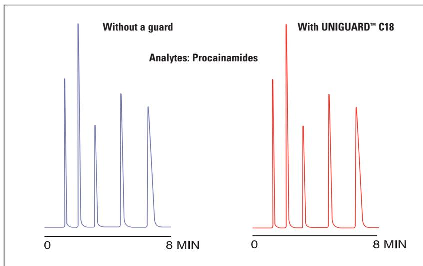
The choice of guard often causes concern. The simple rule of thumb is to choose a guard that is packed with the same particle size and type of material as the analytical column. The guard and column diameters should be as close as possible to eliminate solvent flow and chromatographic discrepancies. A reference table is provided on the left for your convenience.
