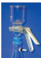
Ideally, all HPLC solvents should be filtered through a 0.45  $\mu$ m filter before use. This removes any particulate matter that may cause blockages. After filtration, the solvents should be stored in a covered reservoir to prevent contamination with dust etc. Filtering HPLC solvents will benefit both your chromatography and the wear and tear of the HPLC system. Pump plungers, seals and check valves will perform better and lifetimes will be maximized.
