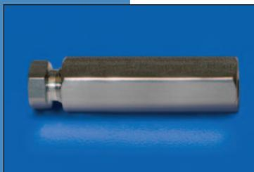
It is advisable to protect your analytical column from sample and system debris and contaminants to maintain the column performance and efficiency. Guard columns or cartridges are one of the most cost effective and efficient ways of trapping these unwanted system components. We recommend a 10 mm length guard for moderate to heavy contamination.
