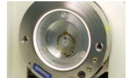
Curtain plate after injection of 25 samples with extractions from raisins without cleanup
