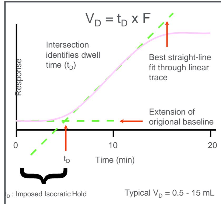
High Pressure Mixing:  $V_D$  = mixing chamber + connecting tubing + injector
