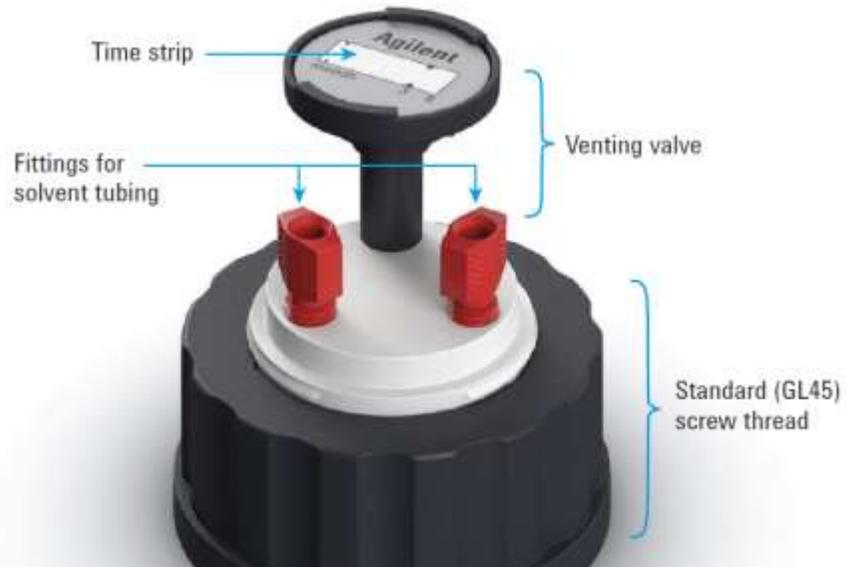
The venting valve plays an important role in maintaining your workspace, keeping it safe and clean. It blocks harmful vapors and assures the required ventilation while solvent is being pulled to the LC instrument.
