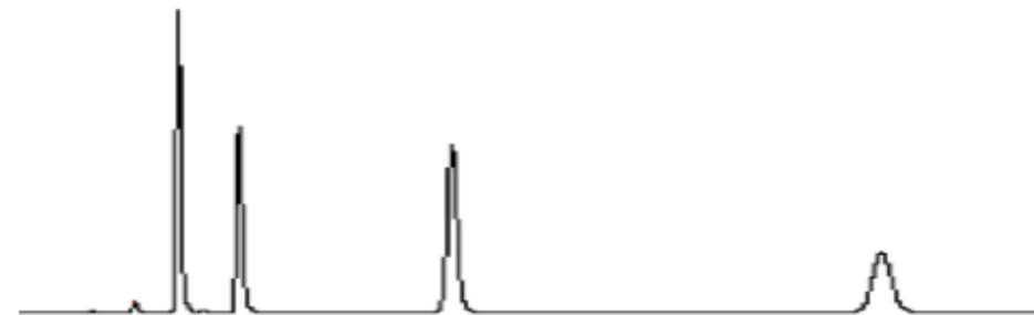
Peak Tailing – Injector Seal Failure
