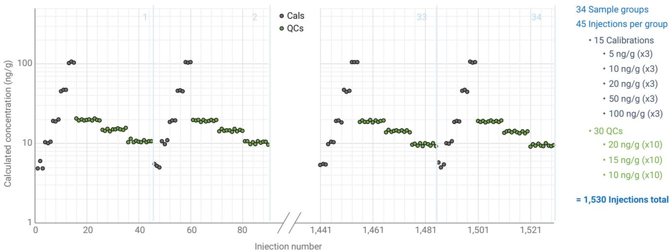
**Figure 3.** Experimental design for quantification repeatability. Calculated concentrations for thiabendazole are plotted for sample groups 1–2 (first 90 injections) and 3–4 (last 90 injections).
