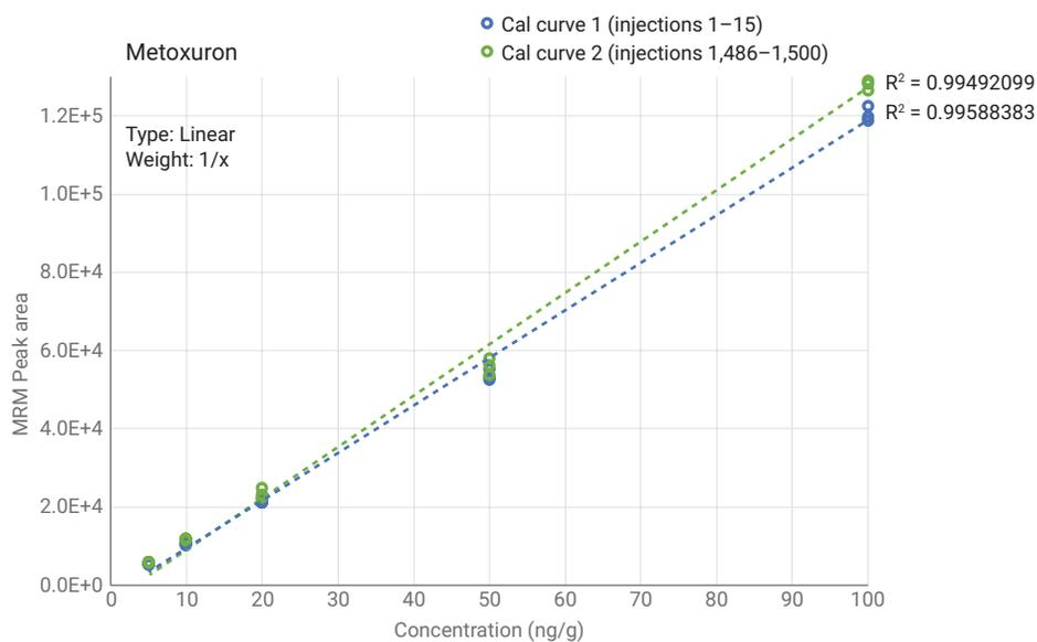
**Figure 4.** Demonstration of accuracy stability. Shown is an overlay of two metoxuron calibration plots corresponding to the first and last sample groups of the 1,530 injections of pesticide-spiked avocado extract.
