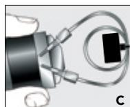
**4** With the IDEX Wrench (page 52), designed especially for fittings, tighten one quarter turn past finger tight. Remove the loop to confirm the ferrule is swaged onto the tube.
