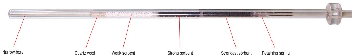
**Figure 1. Design of the focusing trap.** Note the narrow-bore outlet and the long sorbent bed. Sampling occurs from left to right. Desorption occurs from right to left.
