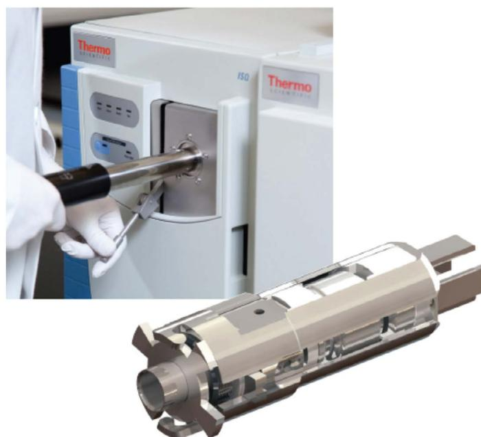
**Figure 11. Schematic of ISQ LT ion source.** Inset shows source being removed with the system under vacuum.
