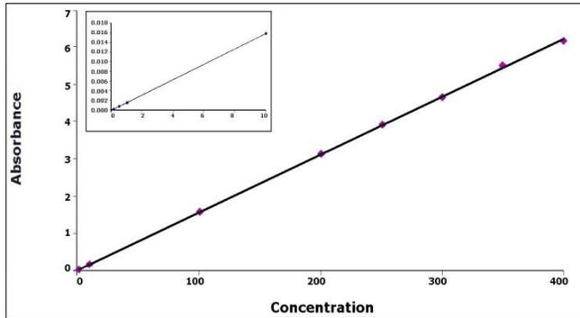
The plot of absorbance vs concentration (mg/L) above highlights the wide dynamic range and inherent linearity ( $r^2 = 0.99988$ ) of the Cary spectrophotometers, and confirms that quantitative analysis of permanganate from 0.1 to 400 mg/L is quite feasible at the peak absorption wavelength of 525 nm up to 6 Abs.
