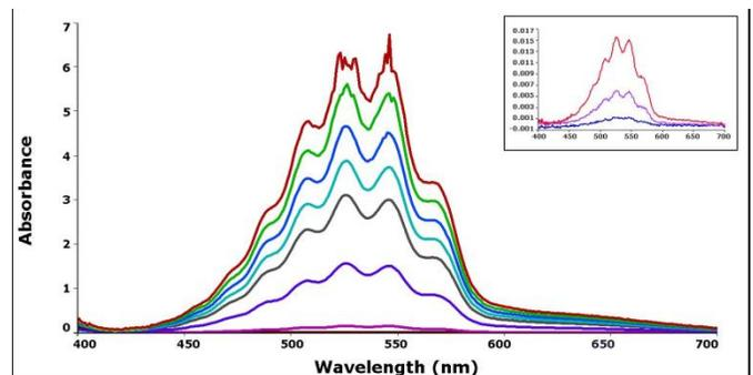
The spectra of standard permanganate solutions can be seen above. The insert shows the spectrum obtained for the lowest concentration standards (0.1 mg/L, 0.5 and 1.0 mg/L), and depicts a spectral profile identical to that of the more concentrated standards.
