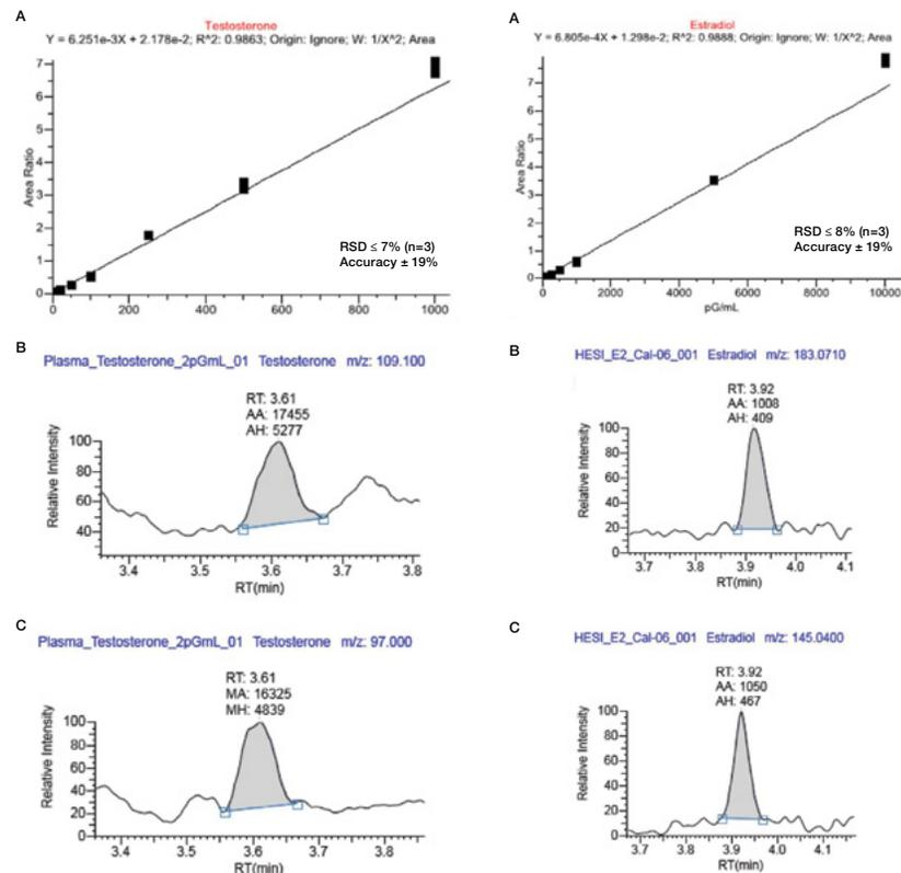
(Left) Testosterone (A) calibration curve, (B) LLOQ chromatogram for quantifying ion, and (C) LLOQ chromatogram for confirming ion. (Right) Estradiol (A) calibration curve, (B) LLOQ chromatogram for quantifying ion, and (C) LLOQ chromatogram for confirming ion.
