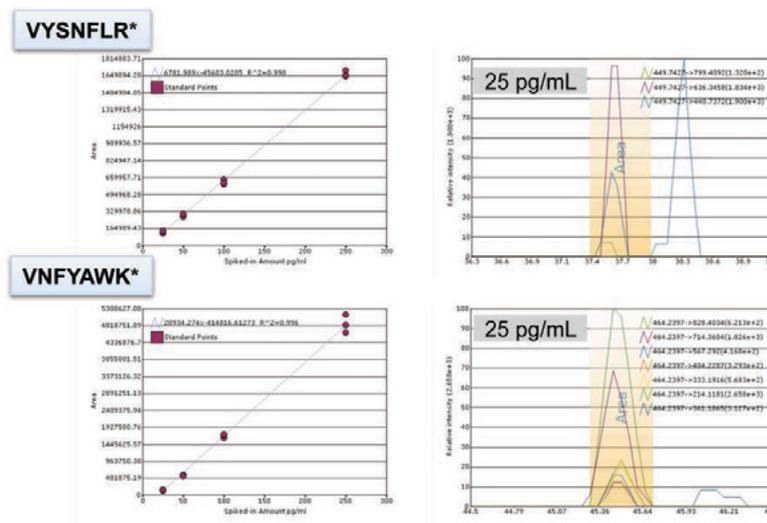
Linearity of the extracted rHuEPO peptides T6 (VNFYAWK) and T17 (VYSNFLR) and extracted ion chromatograms (XICs) of both peptide fragments at the LOD (25 pg/mL) obtained with the Q Exactive mass spectrometer.
