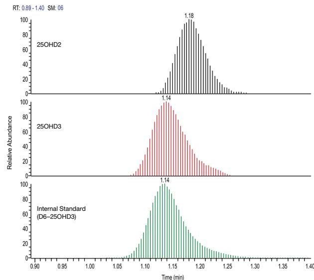
Combined stick mode chromatogram for the internal standard and analytes at their respective LOQs illustrating over 20 scans collected across the peak.
