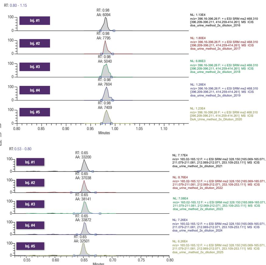
Sensitivity demands of all the analytes were addressed with remarkable ease. As an example, multiple injection profiles of buprenorphine and 6-MAM are shown. The robustness data over five injections were achieved with 1:2 dilution of the urine sample with 2  $\mu$ L injections.
