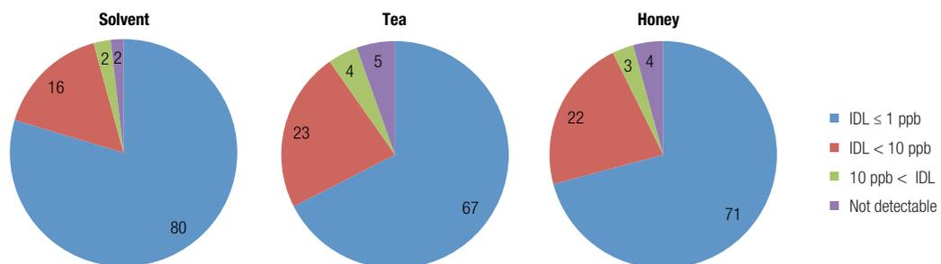
**Relative percentages of different IDL values [ng/g] for the target compounds (328) in solvent, tea, and honey matrices.** More than 85% of target compounds can be detected at ≤10 ng/g, and ~70% of target compounds can be detected at ≤1 ng/g.
