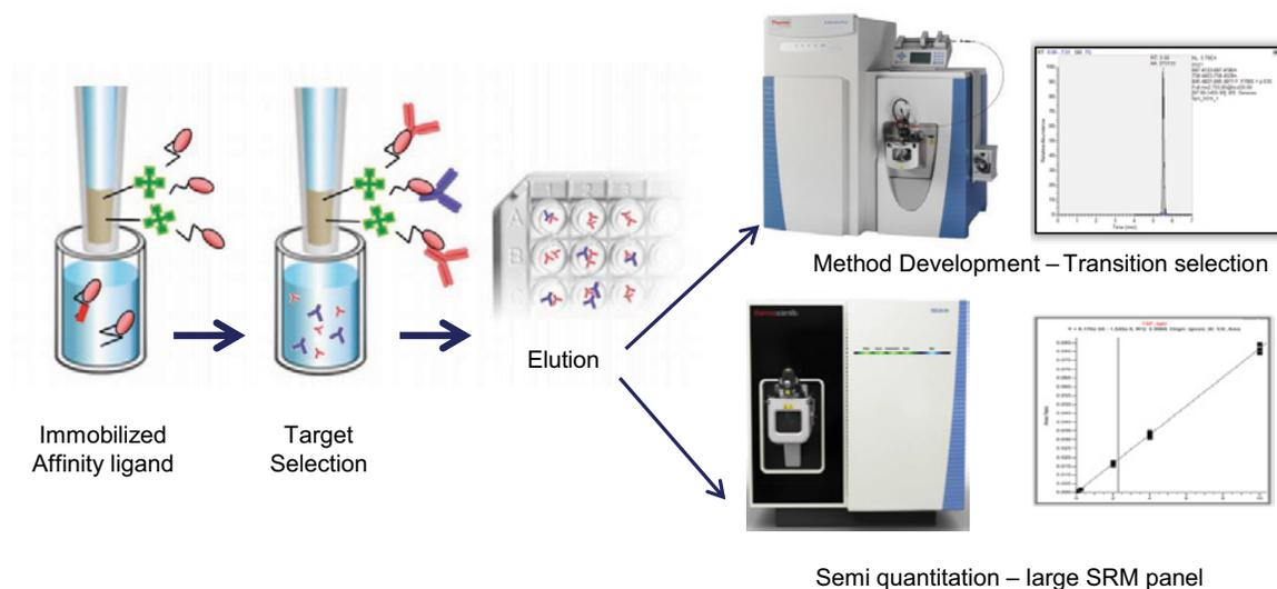
Experimental workflow: MSIA immuno-capture of Tg peptide with detection using capillary LC-MS.
