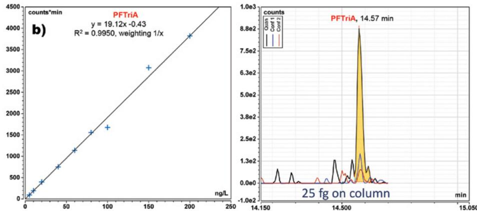
The LLOQs for all 24 PFAS analyzed in this method, based on accuracy and  $RSD \leq 20\%$ , demonstrated the high sensitivity achieved with the TSQ Altis mass spectrometer for the quantitation of PFAS at very low levels (ppt range).
