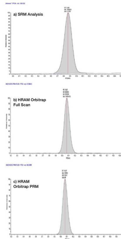
2.5 ppt standard of PFOA analyzed using the Q Exactive mass spectrometer and a triple quadrupole mass spectrometer under similar conditions. Excellent quantitative performance and sensitivity was obtained using the Q Exactive mass spectrometer in both full scan and PRM modes. The results obtained were equal to or better than the published LCMRLs using triple quadrupole SRM methods.
