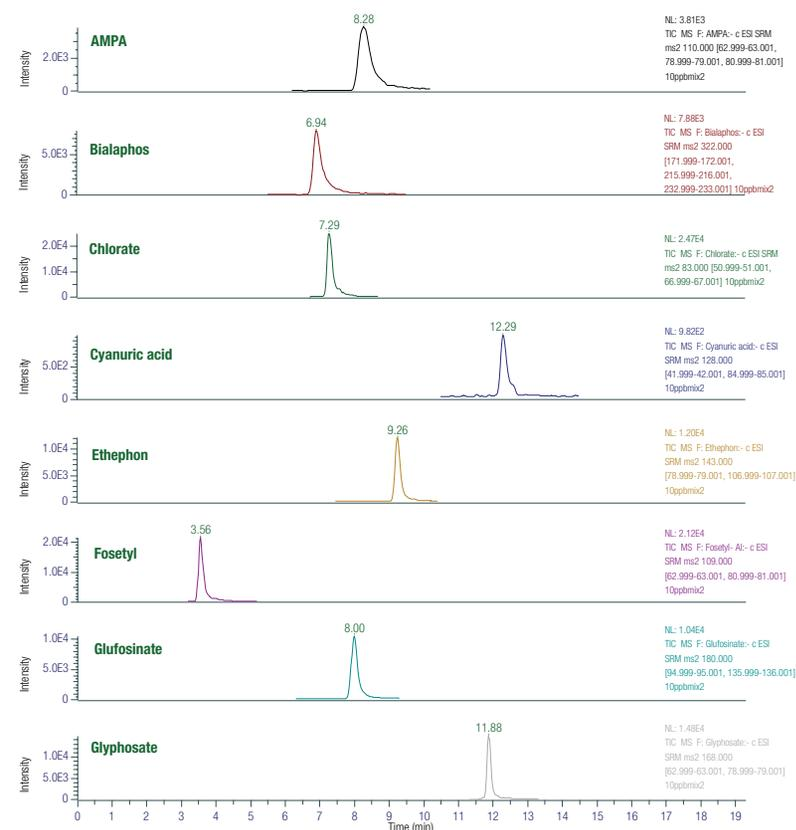
A good IC-MS/MS separation was achieved to resolve 16 analytes in different SRM channels. Fosetyl tends to degrade into phosphonic acid both in solution and in the IC-MS/MS via in-source fragmentation. Phosphonic acid and fosetyl were fully separated on the Dionex IonPac AS19-4 $\mu$ m column with retention times of 8.92 min and 3.56 min, respectively.
