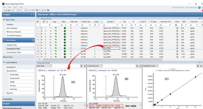
User-defined data processing parameters, including two transitions per analyte, retention time, correlation coefficient, and residuals, were set in the TraceFinder software master method and the data processed automatically. Color-coding flagged whether results passed or failed acceptance criteria. The results that passed user-defined criteria (SANTE guidelines) are shown in green.
