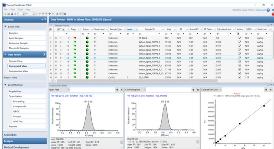
Identification of ametryn in wheat grain was demonstrated with two transitions 228.1→186.1 (quantitative) and 228.1→96.0 (confirmatory) at the same retention (5.85 min,  $\pm 0.1$ ) with ion ratios of 17.23% (11.71–21.76%) observed in wheat grain in comparison with a neat standard. For the quantitative approach, the linearity provided correlation coefficient >0.999 with <15% residuals.
