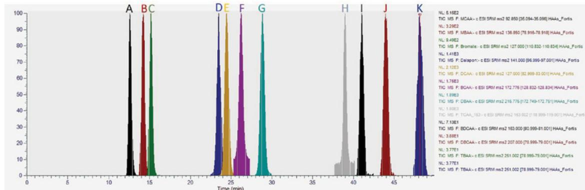
Ion chromatograms of HAAs: (A) MCAA, (B) MBAA, (C) Bromate, (D) Dalapon, (E) DCAA, (F) BCAA, (G) DBAA, (H) TCAA, (I) BDCAA, (J) DBCAA and (K) TBAA at 1 µg/L.
