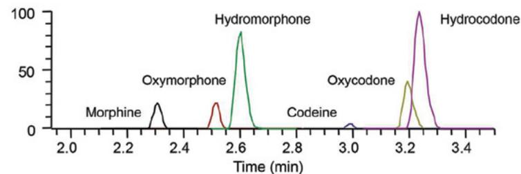
Chromatograms extracted from MS<sup>2</sup> spectra obtained from a confirmation PRM experiment for six opiates at their respective LOQs (2.5 ng/mL for codeine, oxycodone, and oxymorphone, and 5 ng/mL for hydrocodone, hydromorphone, and morphine) in hydrolyzed and diluted urine.
