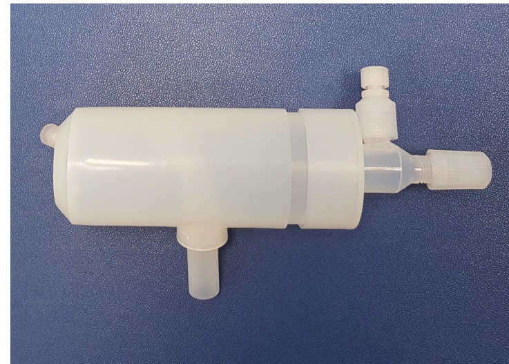
Figure 1. Elemental Scientific PFA barrel spray chamber.
