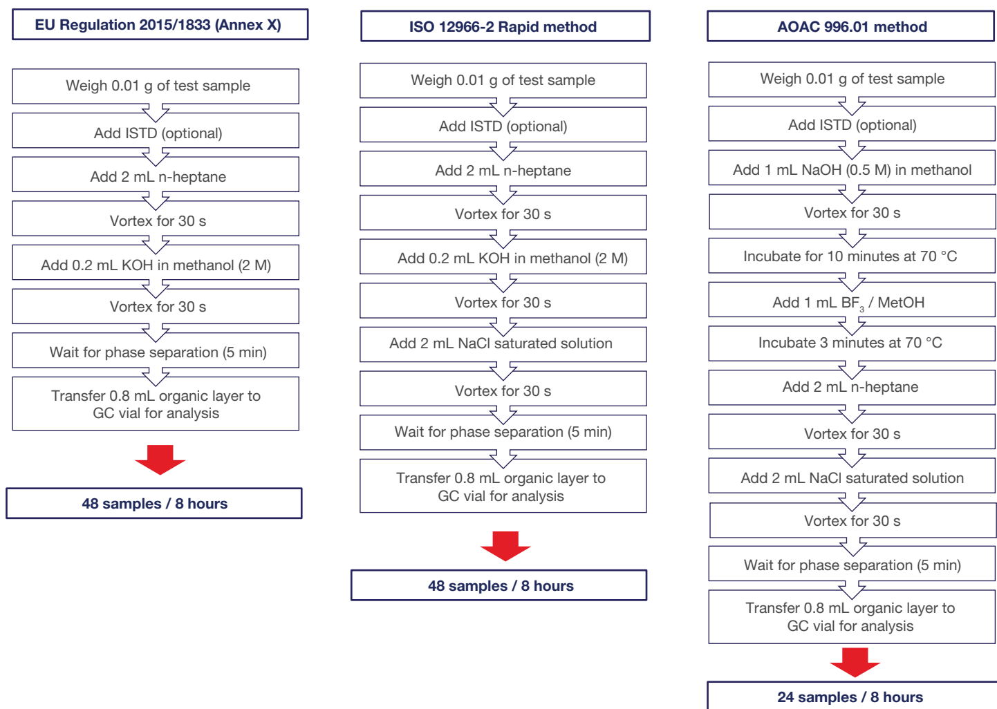
Figure 2. Workflow showing the automated sample preparation according to the EU Regulation 2015/1833 (Annex X), the ISO 12966-2 “rapid” method, and the AOAC 996.01 procedures for fatty acid esterification
