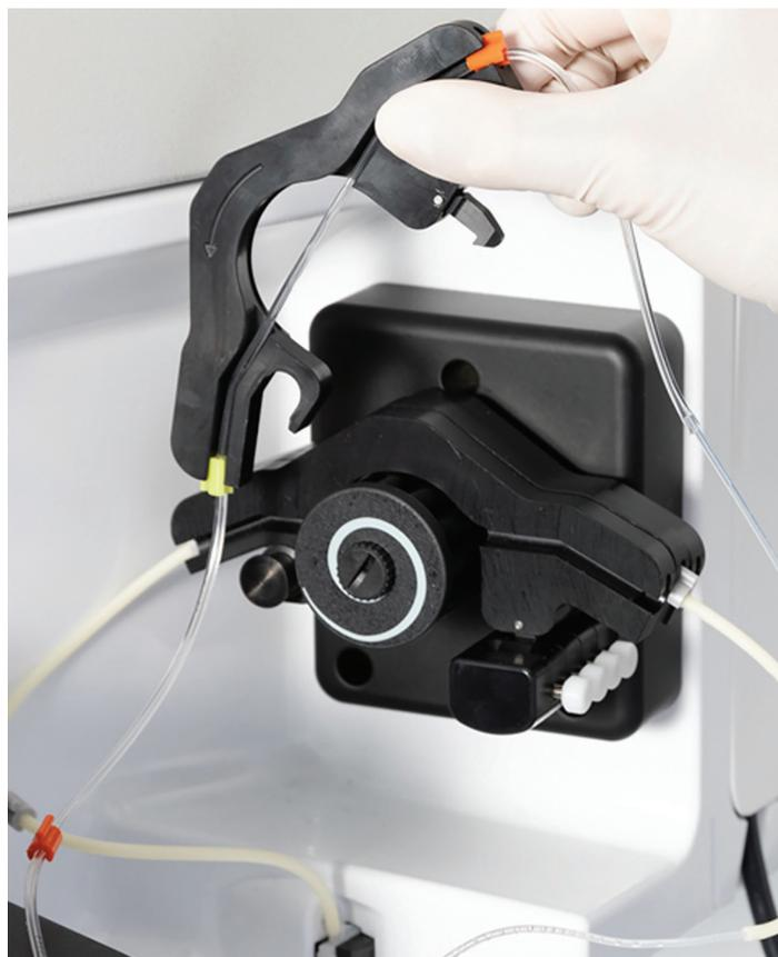
Figure 2. The peristaltic pump (EasyClick) of the iCAP RQplus ICP-MS
