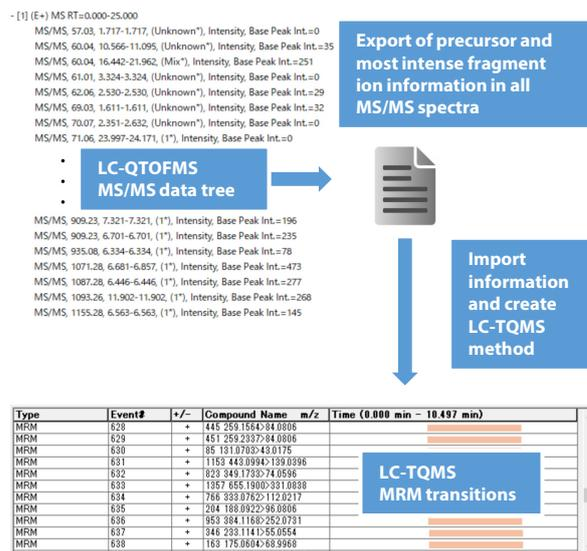
Fig. 2 Automatic Generation of MRM Transitions for LC-TQMS
