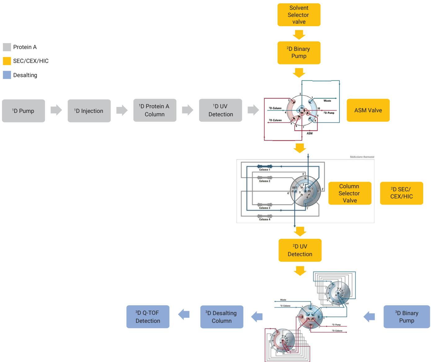
**Figure 1.** 3D-LC/MS configuration incorporating <sup>1</sup>D Protein A separation, <sup>2</sup>D SEC/CEX/HIC, and <sup>3</sup>D SEC-MS-based desalting.
