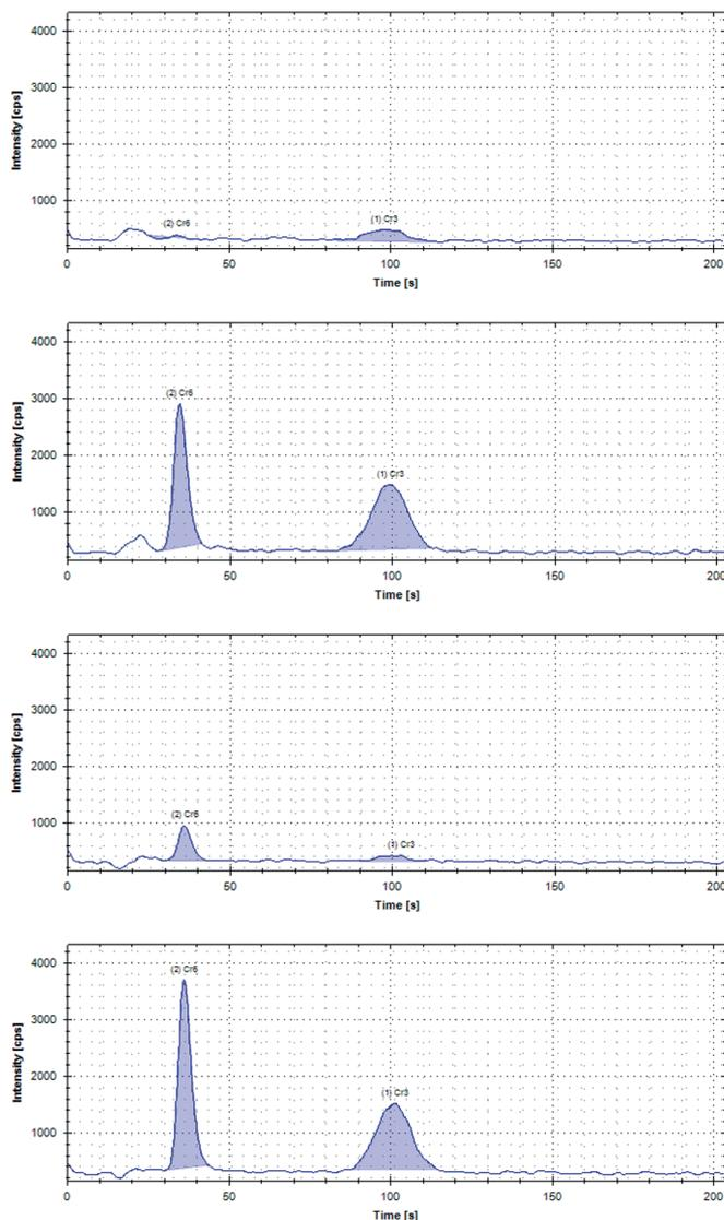
**Figure 1. Chromatograms showing the injection of (from top to bottom) a blank, a standard solution containing  $0.1 \mu\text{g}\cdot\text{L}^{-1}$  of both species (top), tap water, and spiked tap water ( $0.1 \mu\text{g}\cdot\text{L}^{-1}$ ). For better comparability, all are scaled identically.**
