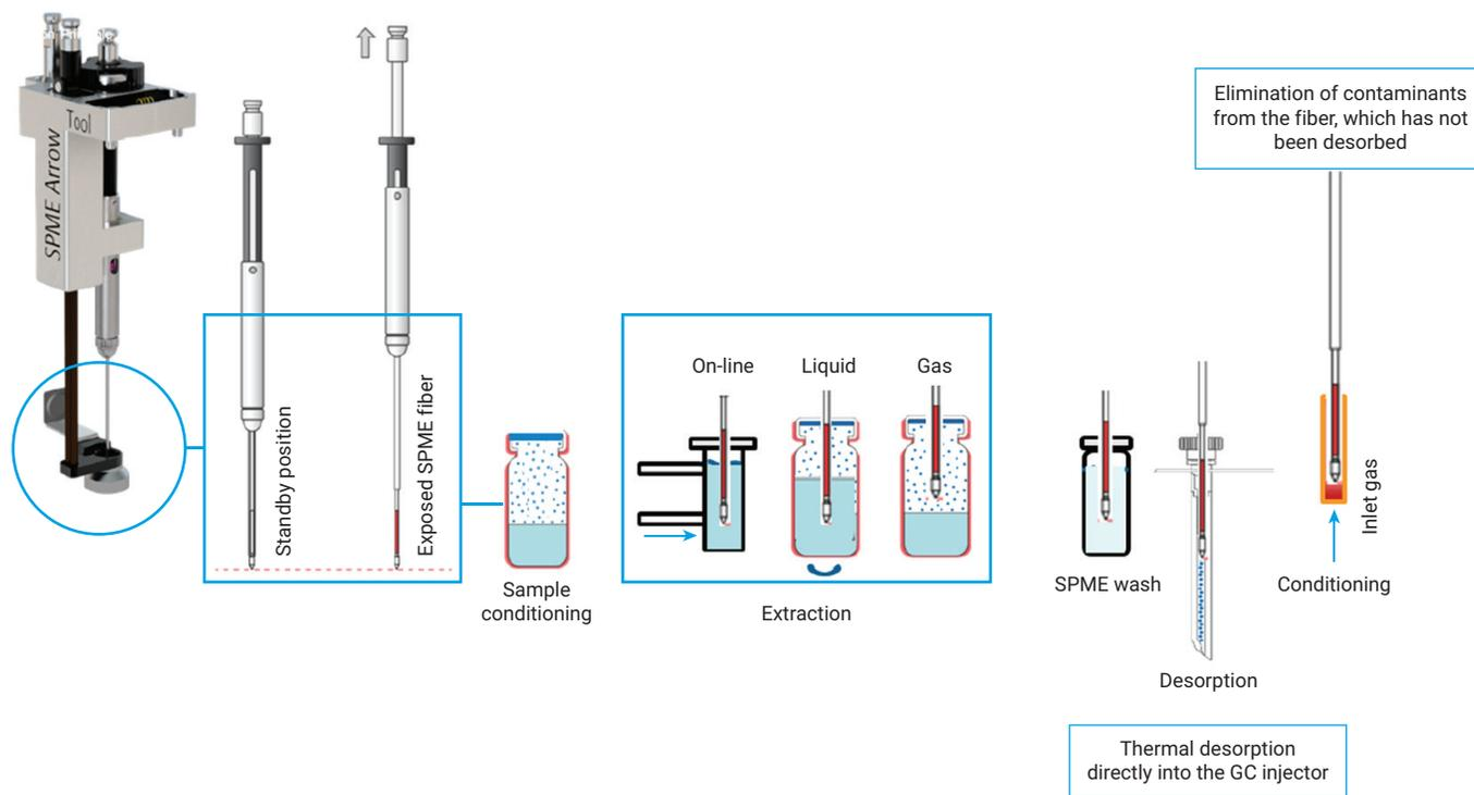
**Figure 2.** Schematic of SPME/SPME Arrow.
