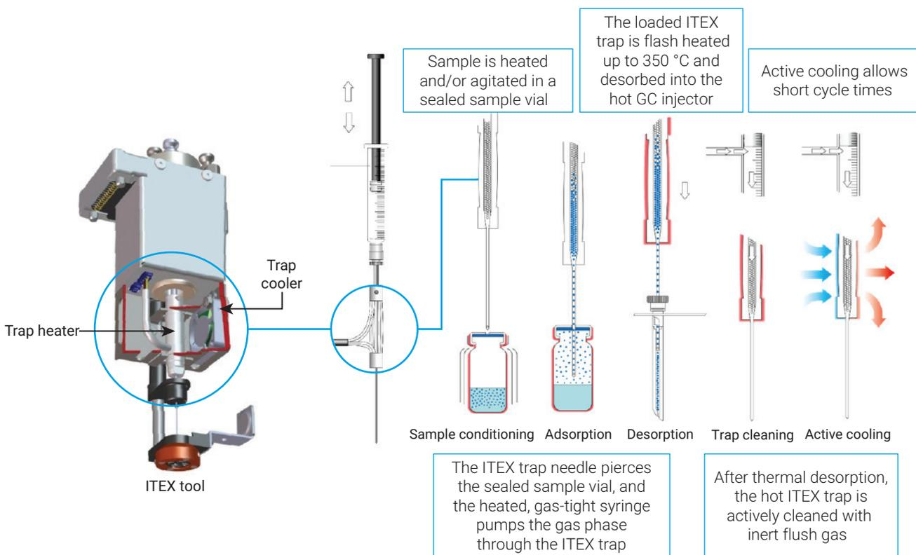
Figure 1. Schematic of dynamic headspace ITEX.
