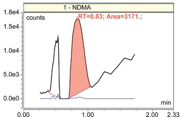
**Figure 4. Mass spectrum of ranitidine drug tablet showing co-elution of NDMA and DMF, which could cause overestimation of NDMA when inadequate mass tolerance setting was used for data processing.** a) Spectrum of ranitidine drug tablet sample containing NDMA and DMF with a resolution setting of 120,000; b) overestimation of NDMA when processing the data with mass tolerance set at 25 ppm; the resultant quantitation is 13% higher as compared with results obtained at 3 ppm (Figure 3b).
