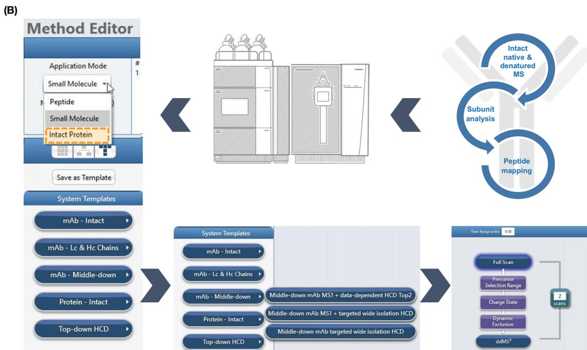
**Figure 2B. Method editor and system templates available on the Orbitrap Exploris 480 mass spectrometer.** A library of pre-defined method templates and an easy instrument setup is provided with the instrument software.
