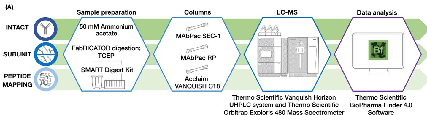
**Figure 2A.** mAb characterization workflows for intact mass analysis, subunit analysis, and peptide mapping comprising sample preparation, separation using suitable column chemistries in combination with liquid chromatography and mass spectrometric analysis, and concluding with software supported data processing
