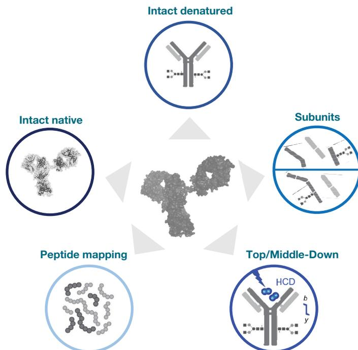
**Figure 1. Complete mAb characterization.** The Orbitrap Exploris 480 MS with BioPharma option supports the complete biopharmaceutical characterization by offering distinct application modes, optimized for the key protein characterization workflows: intact native and denatured, subunit, peptide mapping, and Top/Middle-Down.
