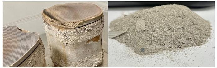
**Figure 1.** Spent car catalysts (left) and partially milled material (right).
