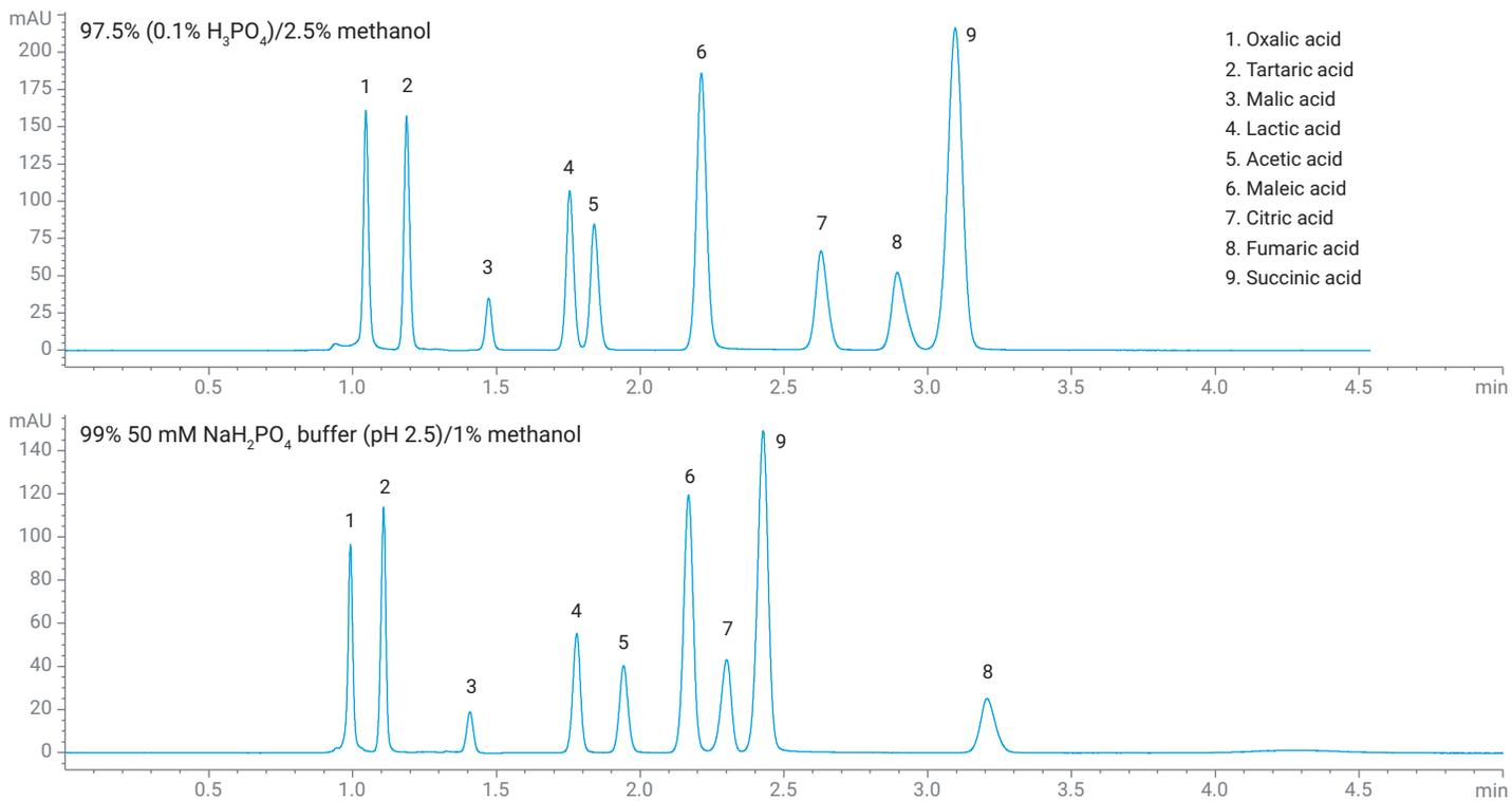
**Figure 1.** Organic acid separation with the Agilent InfinityLab Poroshell 120 Aq-C18 under different mobile-phase additives and compositions.
