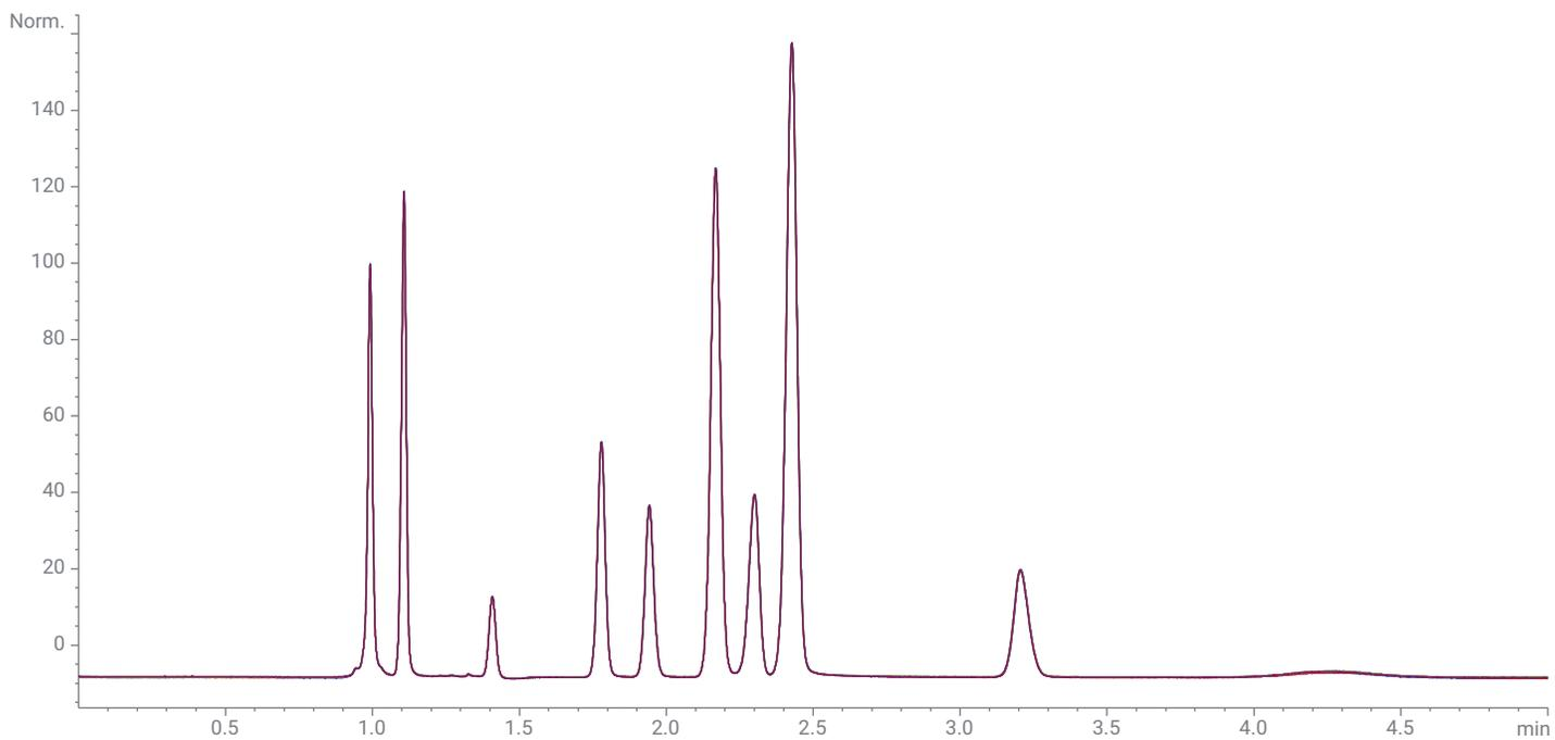
**Figure 2.** Overlay chromatograms of six consecutive injections under 99% phosphate buffer and 1% methanol.
