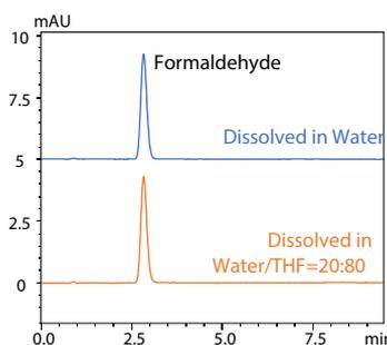
**Fig. 4 Chromatogram of Formaldehyde Standard Solution (1.0 mg/L)**
