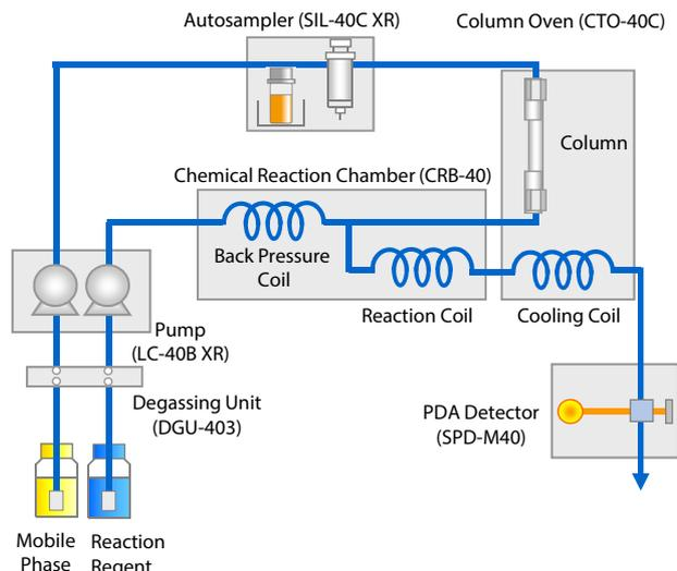
**Fig. 1 Flow Path Diagram of Analytical System**
