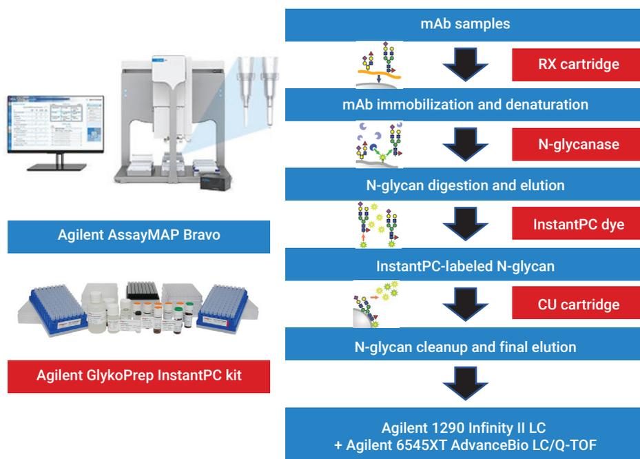
**Figure 1.** Automated N-glycan sample preparation using the Agilent AssayMAP Bravo and Agilent GlykoPrep InstantPC kit.
