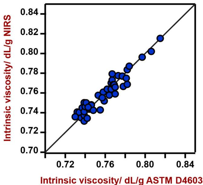
**Figure 3.** Correlation diagram and the respective figures of merit for the prediction of intrinsic viscosity in rPET using a DS2500 Solid Analyzer. The lab value was evaluated according to ASTM D4603.
