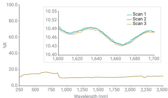
**Figure 4.** Three repeated wavelength scans of PTFE powder acquired at RT using the Agilent Cary 5000 UV-Vis-NIR spectrophotometer. The inset shows the wavelength region between 1,600 and 1,700 nm, highlighting the repeatability of the measurements.
