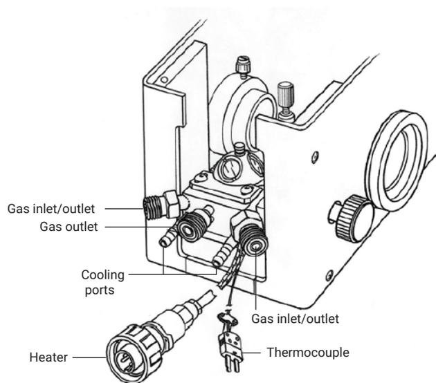
**Figure 3.** The high temperature reaction chamber installed in the Praying Mantis accessory.
