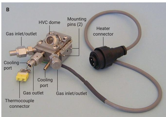
**Figure 2.** (A) Praying Mantis diffuse reflectance accessory. (B) High temperature reaction chamber for the Praying Mantis.
