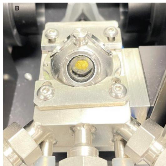
**Figure 6.** (A) Diffuse reflectance spectra of NiSO<sub>4</sub>·6H<sub>2</sub>O measured at 25, 100, and 150 °C. (B) NiSO<sub>4</sub>·6H<sub>2</sub>O converted into a yellow color anhydrous NiSO<sub>4</sub> upon heating.
