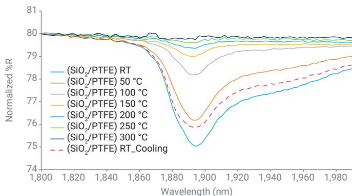
**Figure 5.** Diffuse reflectance spectra of SiO<sub>2</sub> measured at different temperature points from RT to 300 °C. The dotted line represents the trace collected when the sample was allowed to cool down to room temperature.
