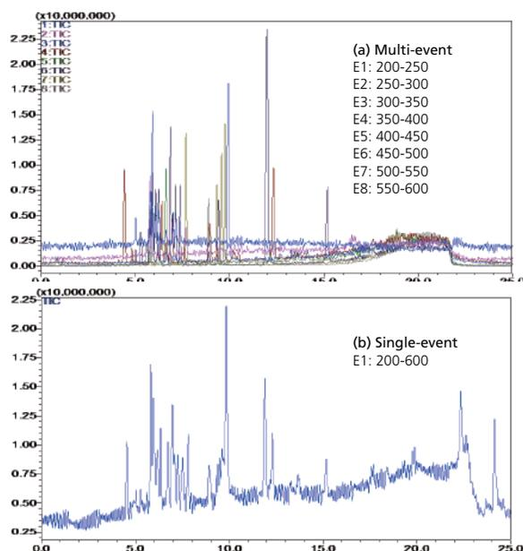
Fig 1: Comparison of TICs of 32 mixed standard of PDE-5 inhibitor drugs and analogues of 0.1ppm acquired by multi-event TIC method (a) and single event TIC method (b).
