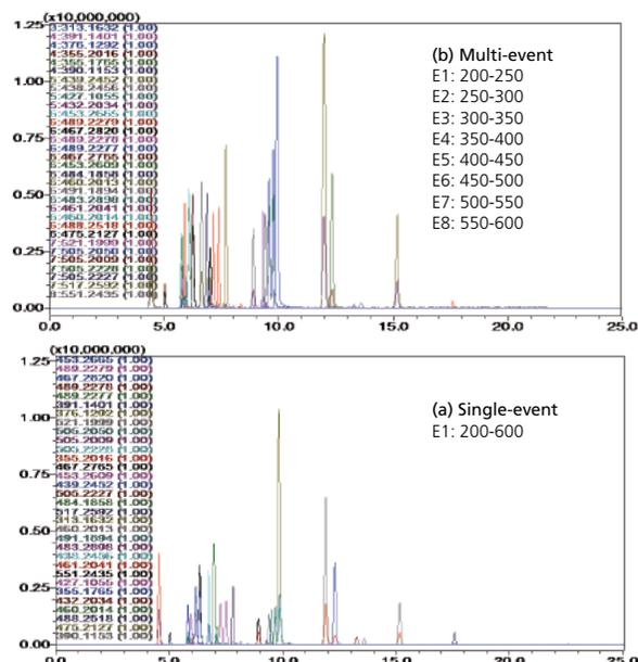
Fig 2: HR-EICs of mixed standard of thirty-two PDE-5 inhibitor drugs and analogues of 0.1ppm acquired by multi-event method (a) and the single event method (b).
