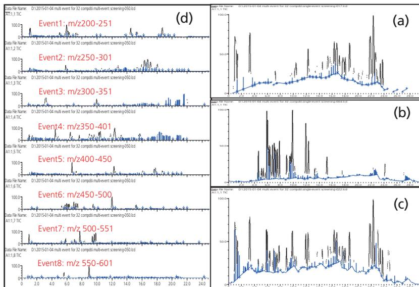
Fig. 4: TICs of spiked 0.5ppm Sample M analysed by multi-event method (d, left) and (a) single event method of blank extract of Sample M, (b) 0.5ppm mixed standards and (c) 0.5ppm spiked Sample M.
