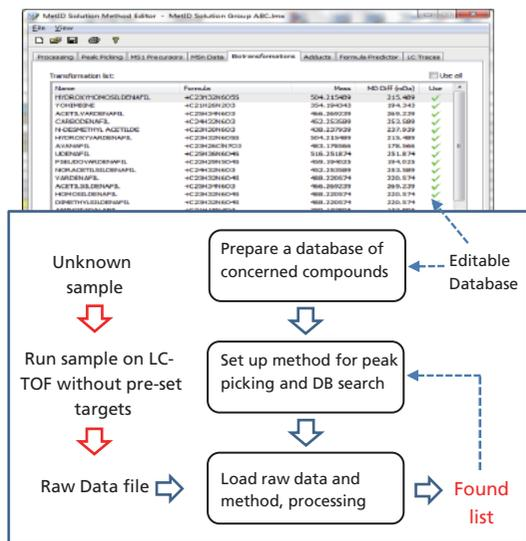
Fig. 3: Un-targeted screening workflow on LCMS-IT-TOF with MetID Solution program for screening analysis of PDE-5 inhibitor drugs and analogues (32 compounds)
