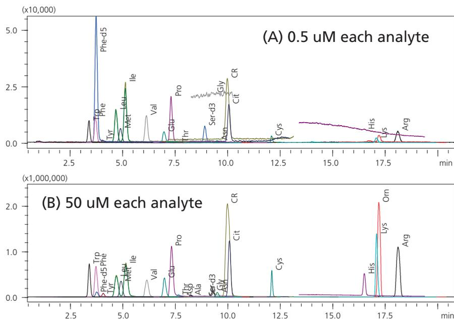
Figure 2: MRM (SIM for Gly) chromatograms of 22 AA and CRE in mixed standards with (5 $\mu$ L inj. volume).
