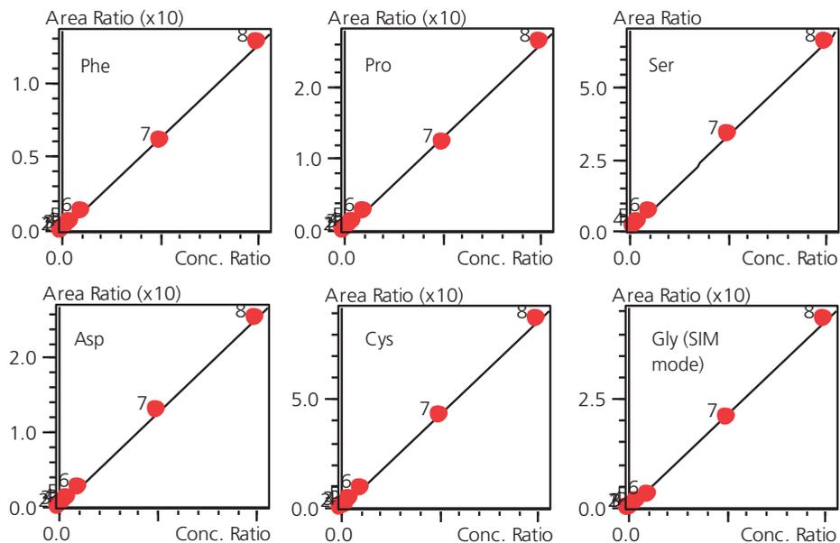
Figure 3: Representative calibration curves of eight levels at from 0.1  $\mu$ M to 100  $\mu$ M on CLAM-LC-MS/MS.
