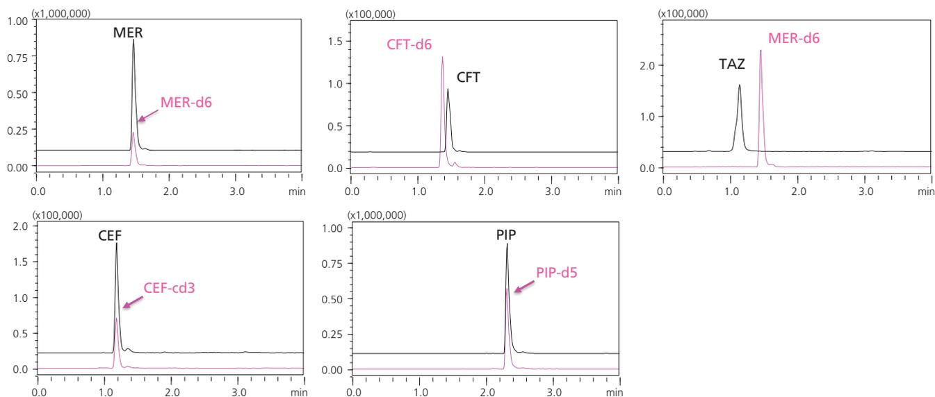
Figure 3: MRM chromatograms of five  $\beta$ -lactam antibiotics each (400 ng/mL) with internal standards in plasma on LCMS-8060
