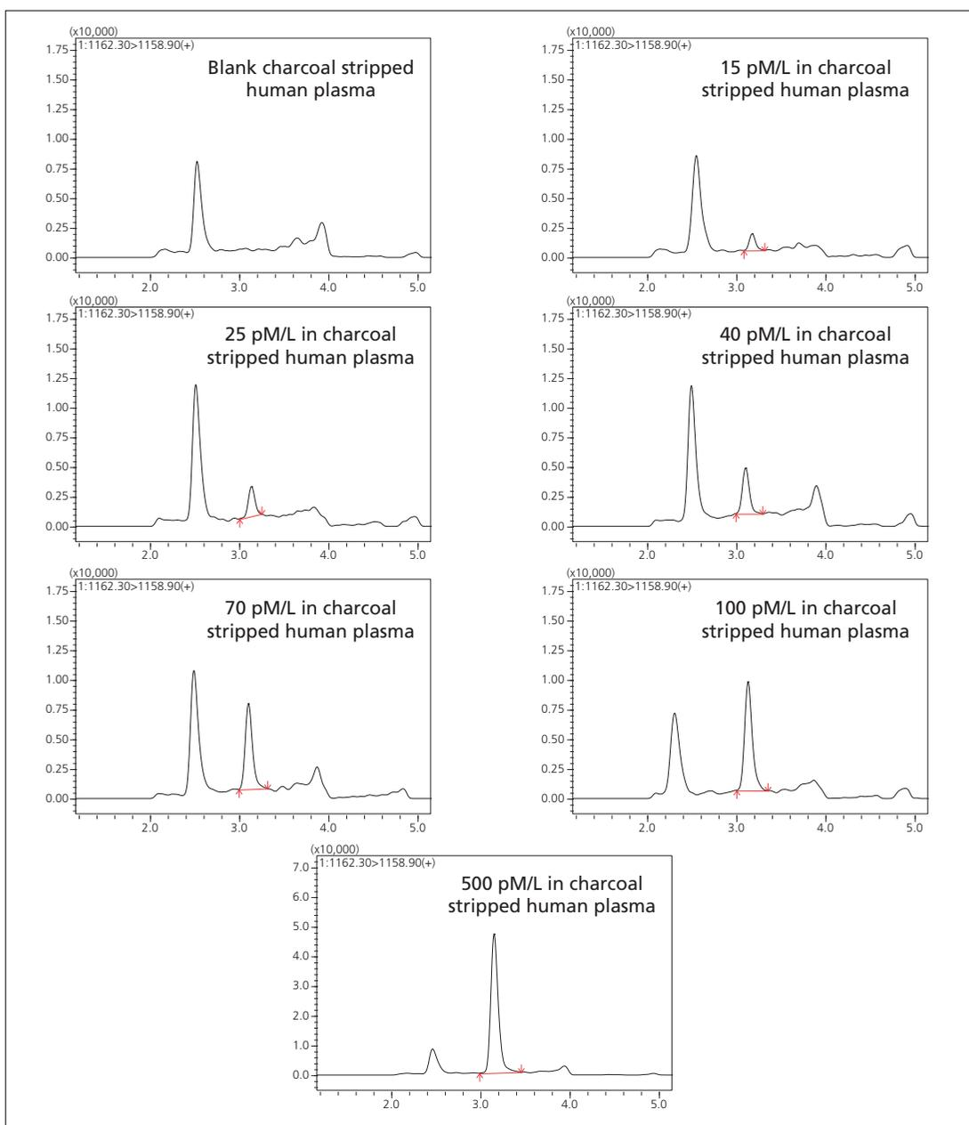
Figure 4. MRM chromatograms of linearity levels for intact human insulin in charcoal stripped human plasma
