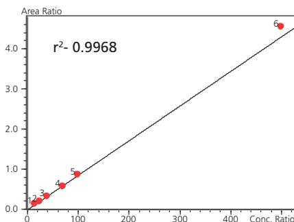
Figure 3. Calibration curve for intact human insulin analysis from charcoal stripped human plasma
