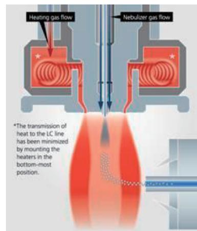
Figure 2. Heated ESI probe
