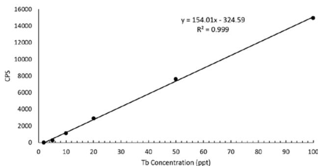
**Figure 1.** Calibration for Tb in the presence of 10 ppm <sup>158</sup>Gd. Tb measured as <sup>159</sup>Tb<sup>16</sup>O<sup>+</sup> by ICP-MS/MS in O<sub>2</sub> mass-shift mode.
