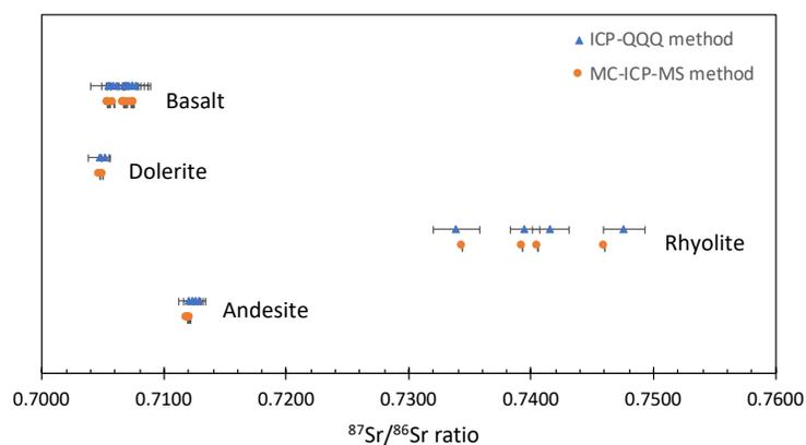
**Figure 3.**  $^{87}\text{Sr}/^{86}\text{Sr}$  IR distribution for typical rocks. Triangle symbol:  $^{87}\text{Sr}/^{86}\text{Sr}$  IR of ICP-QQQ method, error bar in 2SD (n=3). Circle symbol:  $^{87}\text{Sr}/^{86}\text{Sr}$  IR of MC-ICP-MS method, error bar in 2SD (n=3) which falls within the circle mark.
