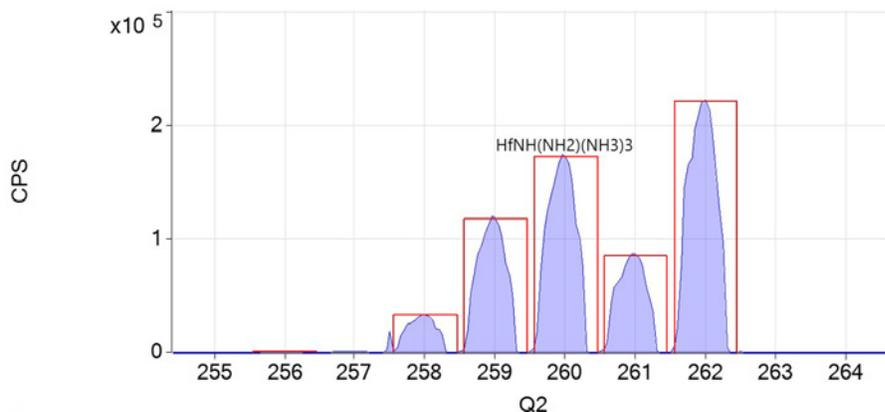
**Figure 4.** Neutral Gain Scan of the Hf isotopes as  $\text{Hf}(\text{NH})(\text{NH}_2)(\text{NH}_3)_3^+$  clusters; theoretical Hf isotopic abundances are shown in red, confirming that the isotope ratios are preserved in the product ion spectrum.
