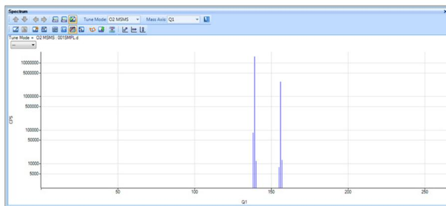
**Figure 3.** Precursor ion scan from 2-260 u for product ion mass 156, in a 50 ppm La matrix. Six peaks are seen at  $m/z$  = 138, 139, 140, 155, 156 and 157, with the intense peaks at  $m/z$  139 and  $m/z$  156 being due to  $^{139}\text{La}^+$  and  $^{139}\text{La}^{16}\text{O}^+\text{H}^+$  respectively.
