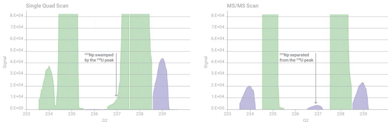
**Figure 1.** Spectrum of  $^{237}\text{Np}$  in presence of 10 ppm U. Left: Single Quad scan and Right: MS/MS mode. MS/MS mode eliminates the peak tail on the low mass side of the intense  $^{238}\text{U}$  peak.
