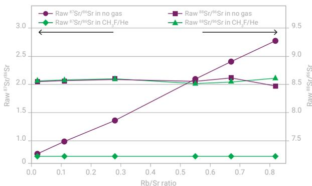
**Figure 2.**  $^{87}\text{Sr}/^{86}\text{Sr}$  and  $^{88}\text{Sr}/^{86}\text{Sr}$  isotope ratios measured using LA-ICP-QQQ in no gas and  $\text{CH}_3\text{F}/\text{He}$  cell gas modes. Reproduced from *J. Anal. At. Spectrom.*, 2016, 31, 464–472 with permission from the Royal Society of Chemistry.
