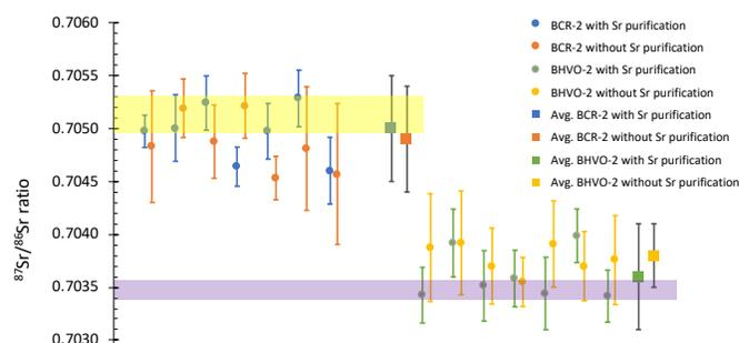
**Figure 2.** Comparison of the measured  $^{87}\text{Sr}/^{86}\text{Sr}$  ratios of BCR-2 and BHVO-2 with and without Sr purification column chemistry by ICP-QQQ with literature values (9) represented by the shaded bands. Circle symbols: average value of each measurement, the error bar is 1SD of the seven replicates of each measurement. Square symbols: the average value of the seven measurements of BCR-2 and BHVO-2, the error bar represents 2SD of the seven measurements.
