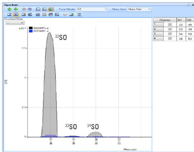
**Figure 1.** Spectra of S isotopes measured in O<sub>2</sub> mass-shift mode. The blank is indicated in blue and the 10 ppb S standard in grey. The spectra show that the BEC of the blank is < 200 ppt.
