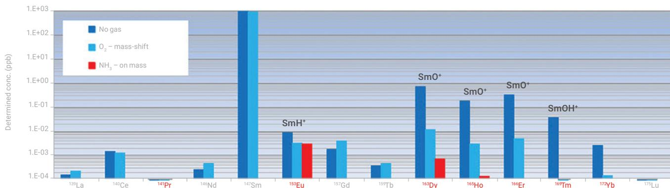
**Figure 2.** Measured concentration of REE impurities in 1 ppm Sm solution. Sm based interferences are observed on Eu, Dy, Ho, Er, Tm and Yb. Only the elements in red were measured in NH<sub>3</sub> on-mass mode.
