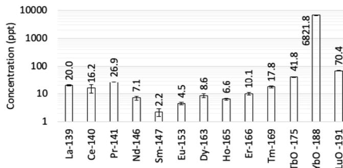
**Figure 2.** Impurity profile and ICP-MS measurement uncertainties (2σ) of Gd<sub>2</sub>O<sub>3</sub> powder used for irradiation.
