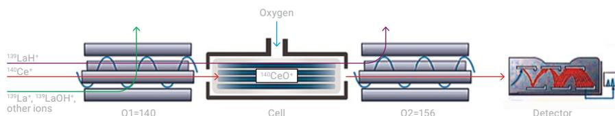
**Figure 1.** MS/MS mass-shift method with O<sub>2</sub> reaction gas; used for the measurement of Ce, as CeO at *m/z* 156, in a La matrix.
