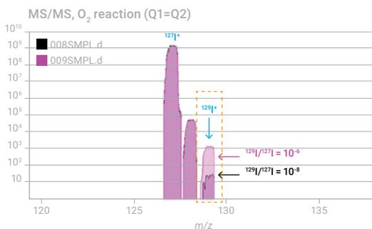
**Figure 2.** Iodine spectra showing both <sup>127</sup>I and <sup>129</sup>I acquired using MS/MS on-mass mode with O<sub>2</sub> cell gas. <sup>127</sup>IH<sup>+</sup> remains to some extent while <sup>127</sup>IH<sub>2</sub><sup>+</sup> is completely removed, as noted later.
