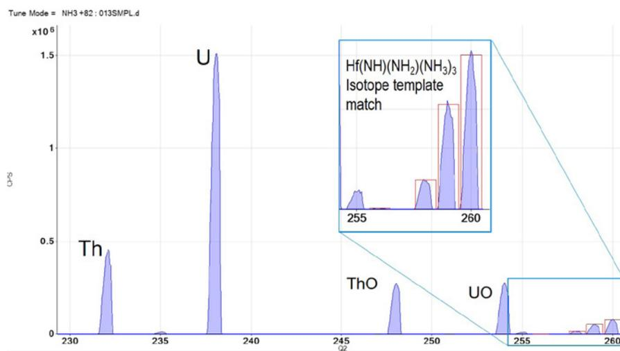
**Figure 6.** Mass spectrum of the mineral sample measured using NH<sub>3</sub> mass-shift mode for Hf and on-mass mode for all other isotopes. The Hf isotopic pattern illustrates that all of the interferences that occurred in Single Quad mode (shown in Figure 5) have been resolved.
