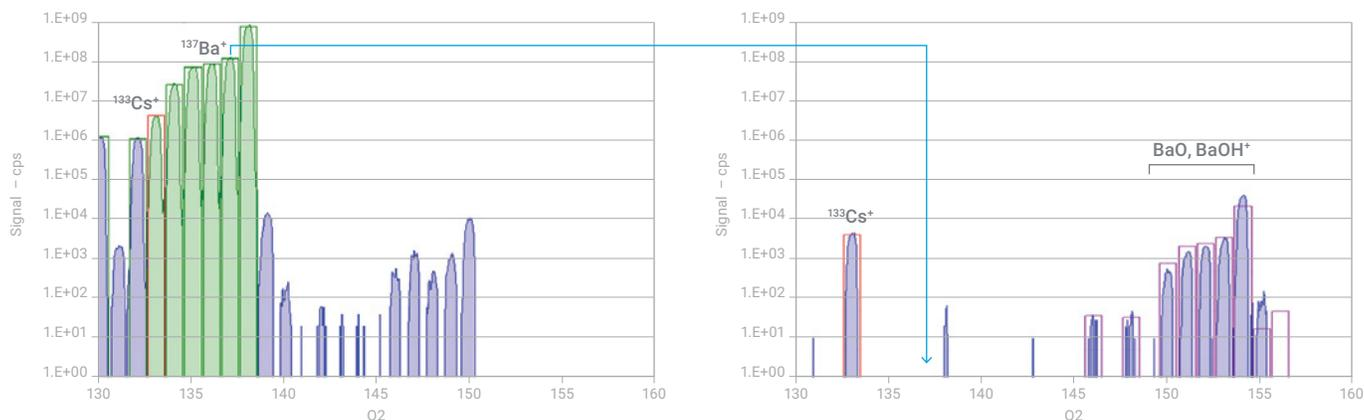
Figure 3. Mass spectra of a solution containing 20 ppb Cs + 5 ppm Ba: (left) SQ no gas and (right) MS/MS N<sub>2</sub>O reaction mode.
