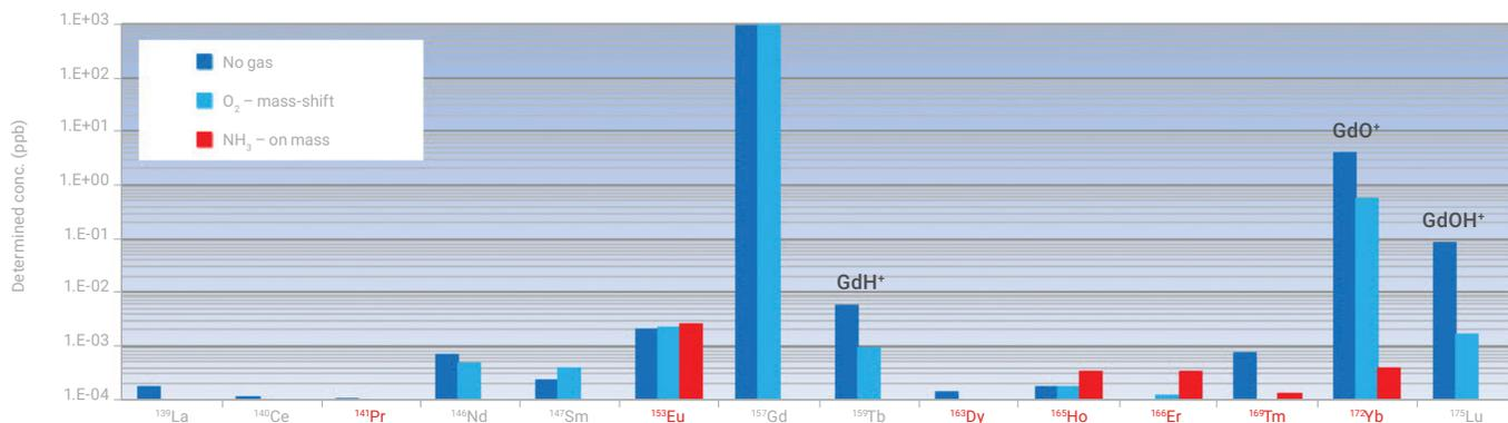
**Figure 1.** Measured concentration of REE impurities in 1 ppm Gd solution. Gd based interferences are observed on Tb, Yb and Lu. Only the elements in red were measured in NH<sub>3</sub> on-mass mode.
