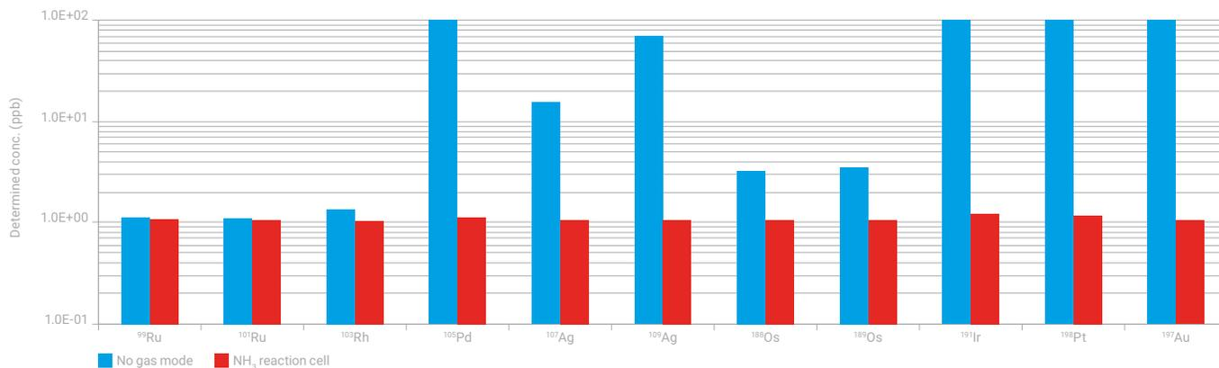
**Figure 1.** Result of synthetic matrix sample test. 1 ppb noble metals were measured in a multi-matrix sample containing 10 ppm of each Cu, Zn, Sr, Rb, Ni, Mo, Pb, Zr, Nb, REEs, Ta, Hf, W and 1 ppm Hg.
