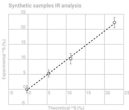
**Figure 2.** Sulfur IR of four synthetic samples.
