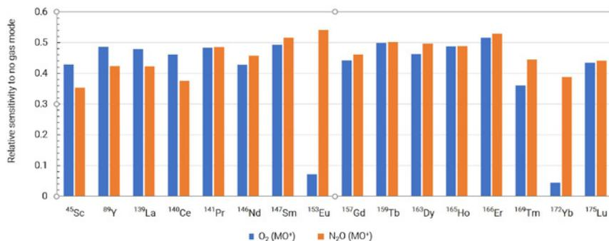
**Figure 1.** Comparison of the sensitivity of ICP-QQQ MS/MS mass-shift method with O<sub>2</sub> and N<sub>2</sub>O cell gas.
