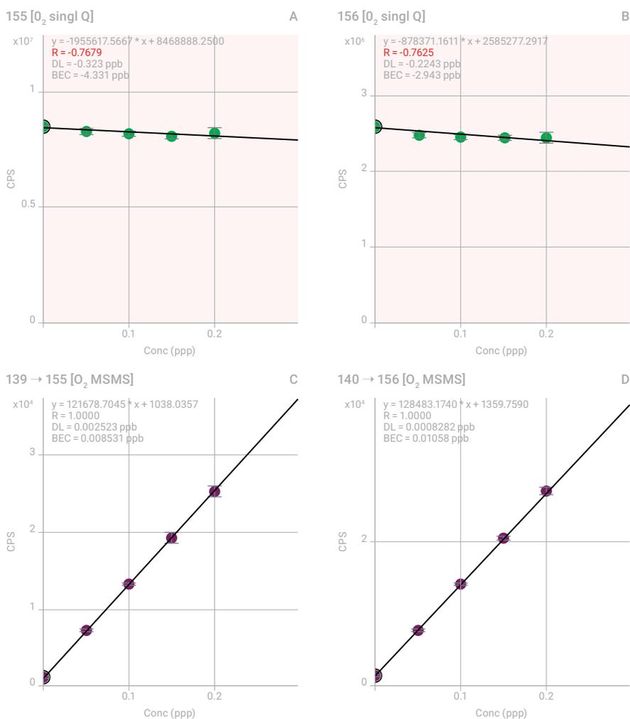
**Figure 2.** Top: Calibration plots up to 0.2 ppb for La in 50 ppm Ba matrix (A) and Ce in 50 ppm La matrix (B), acquired in SQ mode with oxygen reaction gas (emulating conventional quadrupole ICP-MS). Bottom: Calibration plots up to 0.2 ppb for La in 50 ppm Ba matrix (C) and Ce in 50 ppm La matrix (D) acquired in MS/MS mode with oxygen mass-shift.
