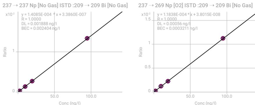
**Figure 3.** Np calibration in a 10 ppm U matrix. Left: no gas mode. Right: O<sub>2</sub> reaction gas mode – showing a 7.5x reduction in BEC. All UH-based interferences were avoided by measuring <sup>237</sup>Np as <sup>237</sup>Np<sup>16</sup>O<sub>2</sub>.
