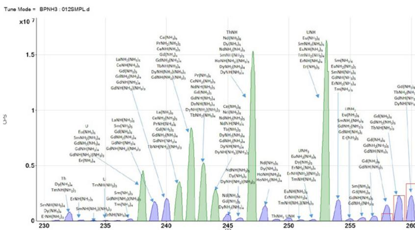
**Figure 5.** Mass spectrum of the mineral sample acquired under Single Quad Bandpass mode using ammonia as the reaction gas. The poor fit of the measured Hf isotopic pattern (far right) illustrates the interferences that occur in Single Quad mode. Some examples of cell-formed ammonia cluster ions are shown.
