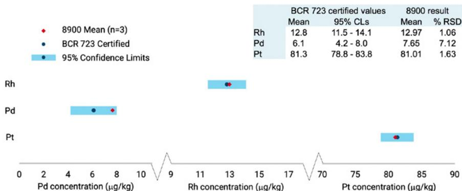
Figure 2. Agilent 8900 ICP-MS/MS measured results compared to certified mean values and uncertainly ranges (95% confidence limits) for Rh, Pd, and Pt in CRM BCR 723 Road Dust.
