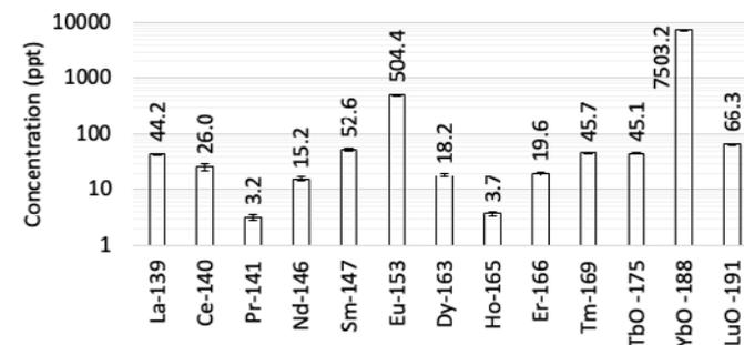
**Figure 3.** Impurity profile and ICP-MS measurement uncertainties (2σ) of a Gd ICP standard using 8800 ICP-QQQ in MS/MS mode with O<sub>2</sub> cell gas.
