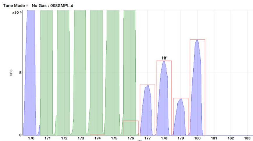
**Figure 1.** Hf (red peak template) in the presence of Lu and Yb matrix. The poor template fit for  $^{176}\text{Hf}$  (highlighted in blue outline) is due to the contribution from  $^{176}\text{Lu}$  and  $^{176}\text{Yb}$  to the signal at  $m/z$  176.
