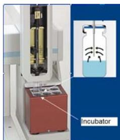
Fig. 1: 20 ml Headspace vial placed into incubator of the AOC-5000
