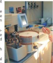
Usually, the cartridge enters into the Turbomatrix tube by simple pouring. If it does not occur, use a pushing tool to press the cartridge till the nick on the tube.
