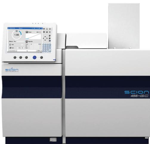
The SCION GC based Natural Gas Analyzer
