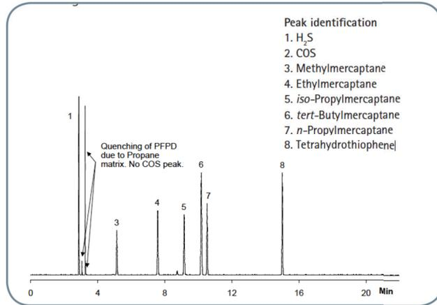
Figure 10a: Sulfur compounds in propane, BR-1 column
