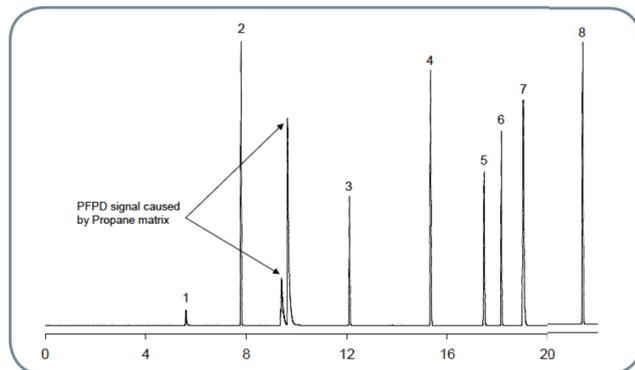
Figure 10b: Sulfur compounds in propane BR-QPLOT column
