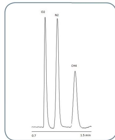
Figure 12c: O<sub>2</sub> and N<sub>2</sub> on GC-1.
