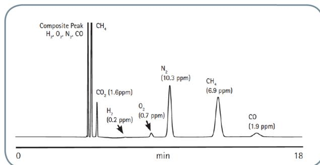
Figure 11: LPG Sample separation
