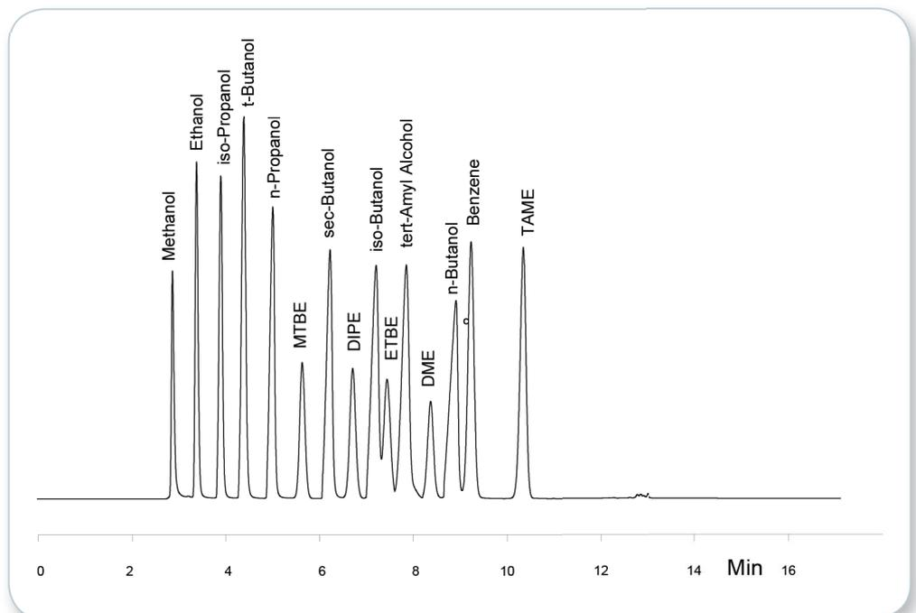
Figure 9. Oxygenate test standard separation
