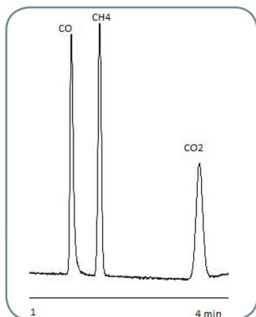
Figure 12a: CO, CH<sub>4</sub> and CO<sub>2</sub> on GC-1.
