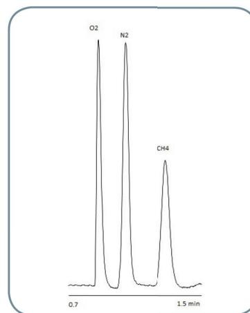
Figure 12c: O<sub>2</sub> and N<sub>2</sub> on GC-1.
