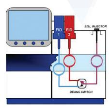
Deans switching enables the use of multiple traps and columns of differing phases in one method/analysis. It is the basis of two dimensional GC and of the many standard analyzers manufactured by Scion Instruments. Use our expertise to configure the optimum system for you.
