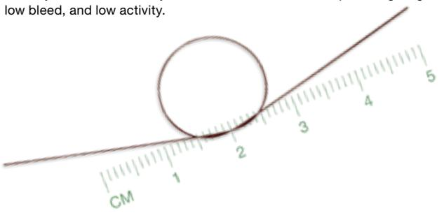
**\*\* Evaluated by performing 185 programmed temperature runs, total 23 hours at 430 °C. Polyimide tubing was still flexible as shown here.**
