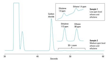
Figure 4. Chromatogram for carbon dioxide, ethane and ethylene on the fourth column channel.
