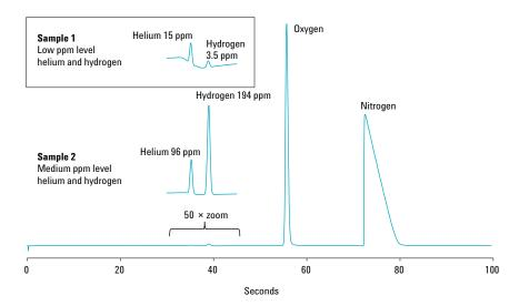
Figure 2. Chromatogram for helium, hydrogen, oxygen and nitrogen separation on the first column channel.
