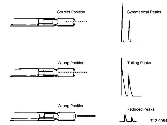
pyrolyze or carbonize both the stationary phase and the column's outer coating, producing a highly adsorptive outlet. In some detectors, transfer lines with right angle turns or very small inner diameters prevent insertion of the column into the detector. Consult the manufacturer about overcoming this problem, perhaps with a part substitution.
