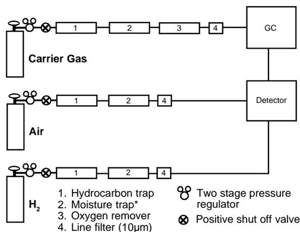
NOTE: The functions of a moisture trap and an oxygen remover are combined in our OMI-2 and High Capacity gas purifiers (see products pages). 712-0083
