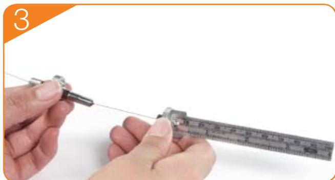
3 Insert the end of the column and column nut into the bottom of the Cool-Lock Nut Installation Gauge.
