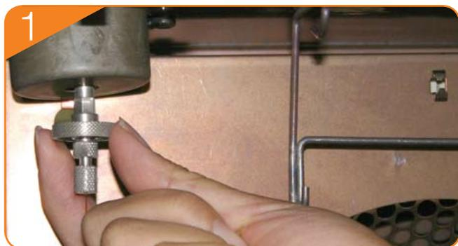
1 Detach the Cool-Lock Nut and column from GC instrument.
