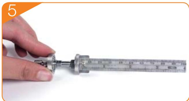
5 Tighten its bottom ferrule. Make sure lower body/ ferrule is in the full extension position.
