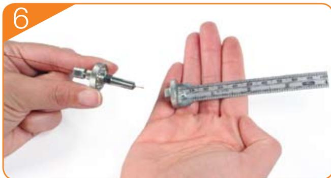
6 Unscrew the installation gauge and install the nut and column into the instrument. Make sure Cool-Lock nut is in the full extension position to achieve the correct premeasured position, and allow for proper leak checking.
