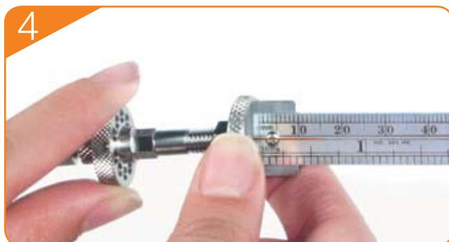
4 Hand-tighten the column nut into the gauge until the ferrule starts to compress. Adjust the length of the column to the desired length. Further tighten the nut into the gauge until the column cannot slide.
