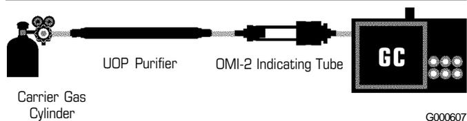
**Figure C. Simple Purifier Configuration for a Single-GC System with Undemanding Requirements**
