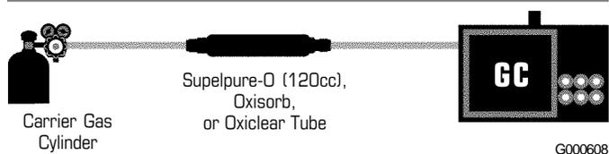
**Figure D. Purifier Scheme for a System with High Purification Demands**
