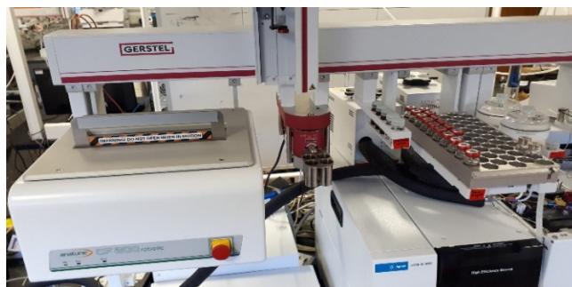
Figure 1: DiLLME set up (Centrifuge, QuickMix and sample tray with High recovery Vials)
