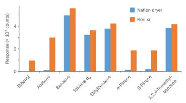
Kori-xr shows enhanced recovery of low-boiling and polar VOCs from an air stream with 80% RH, compared to use of a Nafion™ dryer.
