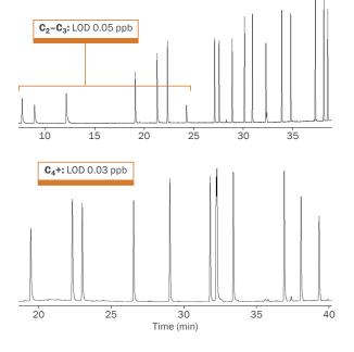
The efficient operation of the Air Server-xr provides limits of detection (LODs) well below the 0.5 ppb required, for ozone precursors ranging from acetylene to trimethylbenzene.
