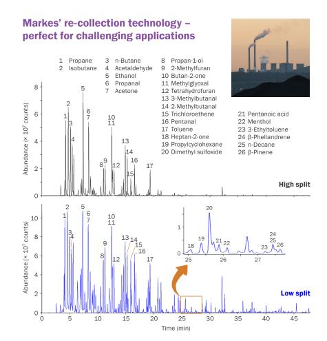
Markes' sample splitting and re-collection technology allows samples such as this odorous industrial air to be re-analysed. As well as aiding method validation and offering greater peace-of-mind, it also allows a single sample to be analysed at different split ratios, allowing both high-and low-concentration components to be accurately quantitated.
