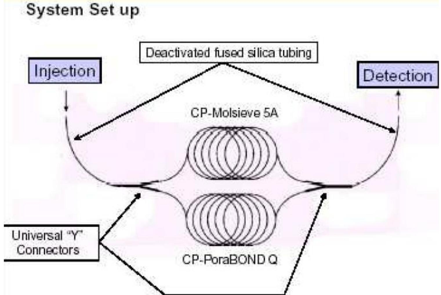
**Set-up for Select Permanent Gases/CO<sub>2</sub>**
