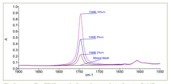
The Spectrum Two FT-IR provides fast and easy analysis of varying FAME concentrations in diesel fuel.
