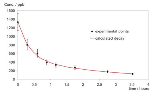
Decay of mesitylene in a volunteer's breath after a two-hour controlled exposure, measured using SIFT-MS. The solid line represents a two-reservoir fit to the experimental points
