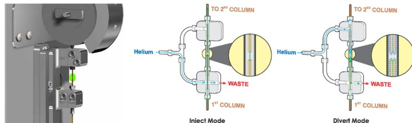
Figure 1. Diagrams showing LECO's Pegasus BT FLUX modulator and its modes of operation
