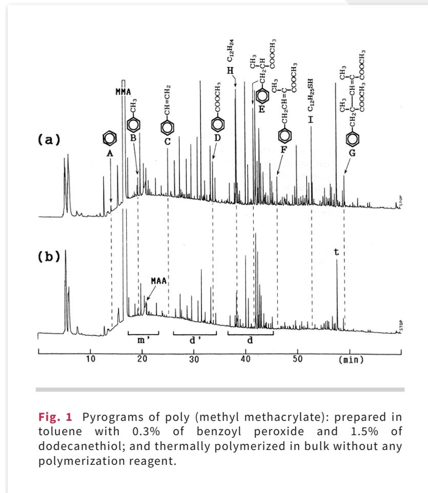
**Fig. 1** Pyrograms of poly (methyl methacrylate): prepared in toluene with 0.3% of benzoyl peroxide and 1.5% of dodecanethiol; and thermally polymerized in bulk without any polymerization reagent.
