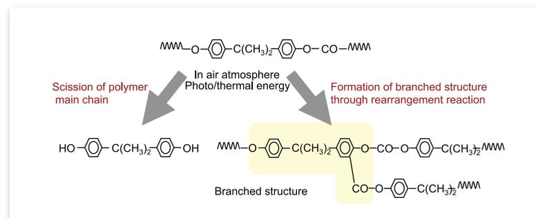
**Fig. 2** Expected photo/thermal/oxidative degradation reactions of PC
