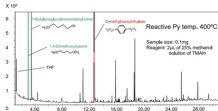
**Fig. 2** Pyrogram obtained by reactive pyrolysis of PBT
