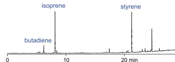
**Fig. 1** Fig. 1. Pyrogram of a blend rubber
