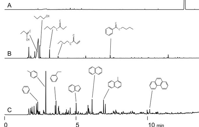
**Fig. 2** Chromatograms of temperature zones of EGA thermogram
