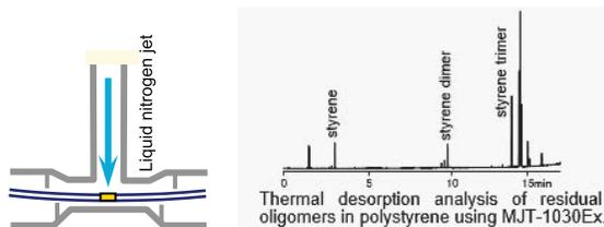
Thermal desorption analysis of residual oligomers in polystyrene using MJT-1030Ex.
