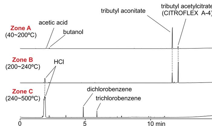
**Fig. 2** Chromatograms for zones A through C by Heart-Cutting EGA-GC/MS method
