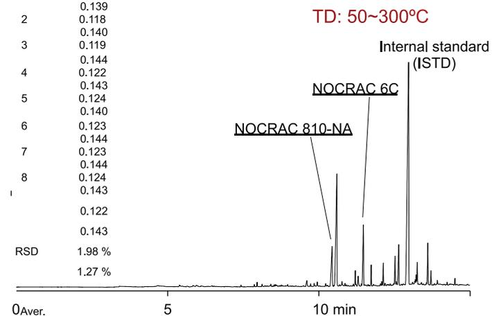
**Fig. 2** Chromatogram for Zone A by (TD)-GC/MS analysis
