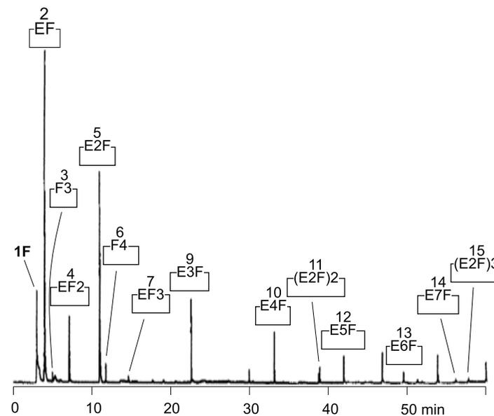
**Fig. 1** Pyrogram of copolyacetal by reactive pyrolysis
