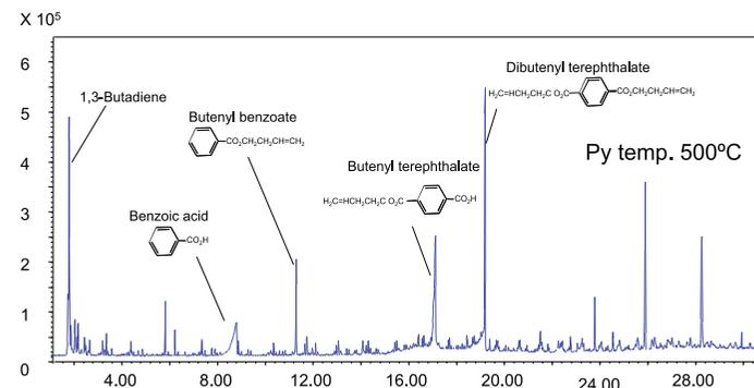
**Fig. 1** Pyrogram obtained by flash pyrolysis of PBT
