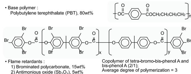
**Fig. 1** . Base polymer and structure of flame retardant
