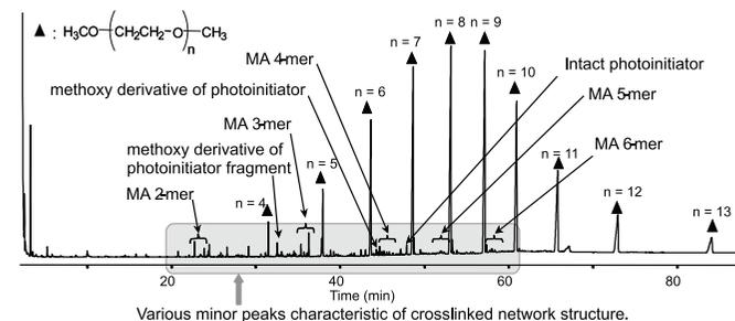
**Fig. 1** Typical pyrogram of UV-cured resin prepared from polyethyleneglycol diacrylate and morpholino-type photo-initiator. Pyrolysis temp.: 400°C, GC oven temp.: 35°C (6 min)-(5 °C/min)-340°C Separation column: Poly(5% diphenyldimethylsiloxane), L=30 m, id=0.25 mm, df=0.25 µm
