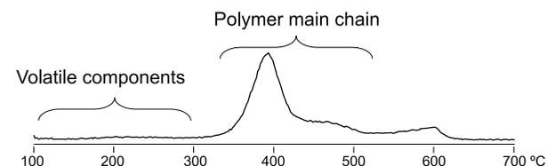
**Fig. 1** Evolved gas curve of a compounded rubber
