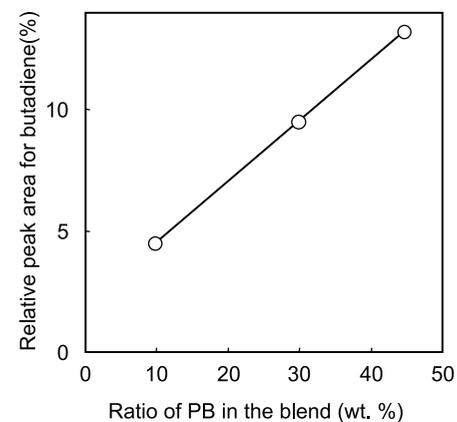
**Fig. 2** Calibration curve for PB in the blend
