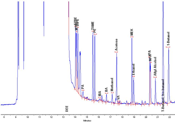
Chromatogram: oxygenates free gasoline spiked with 100 ppm calibration standard
