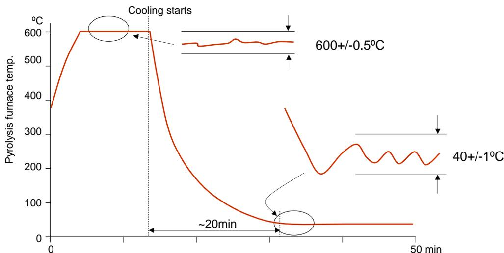
Fig. 2 Temperature Profile of Pyrolysis Furnace
