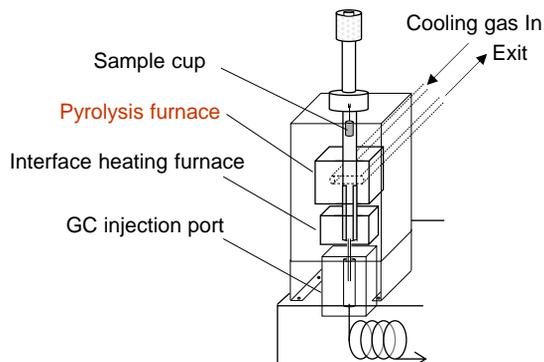
Fig. 1. Structure of Double-Shot Pyrolyzer
