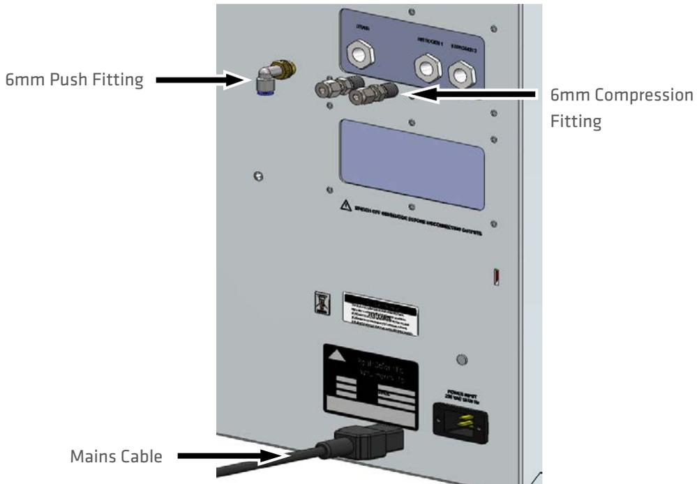
Figure 3: Rear Connections
