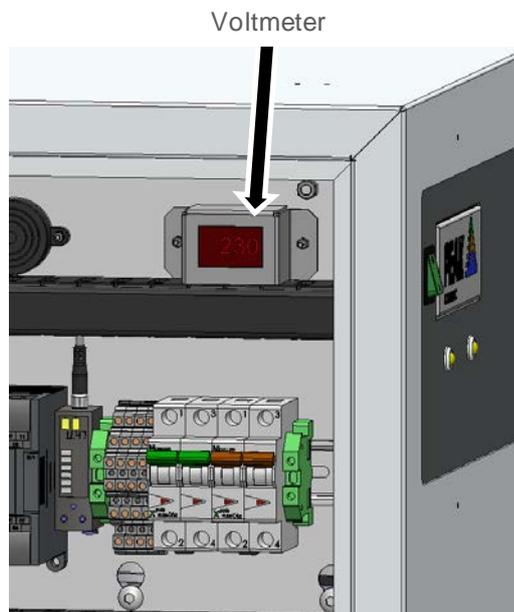
Figure 4: Voltmeter Location
