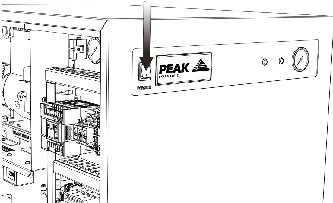
Switch the generator power **ON** using the switch on the front panel.
