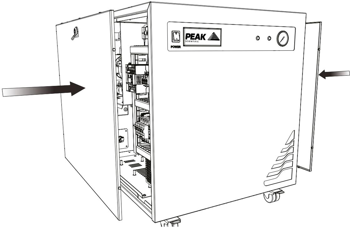
Re-attach both side panels to the generator, ensuring the **earth leads** are **re-connected** and the **locks** are **secured**.
