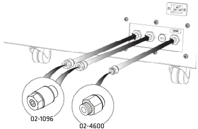
Select the **1/4"- 6mm Push Fit Fitting 02-4600** and attach to the Drain port at the rear of the generator. Attach the **Flow Control Silencer(s) 02-1096** to the remaining port(s).
