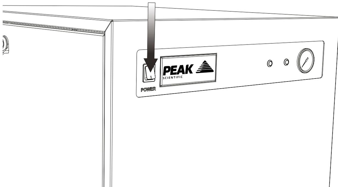
Switch the generator power **ON** using the switch on the front panel.
