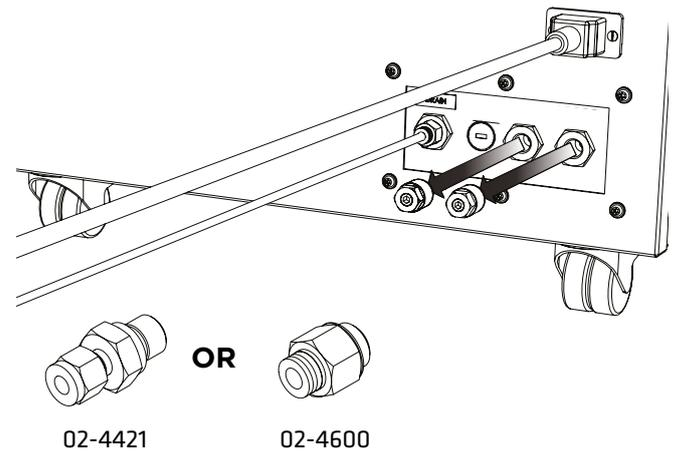
Depending on the size of the inlet on the instrument, select either the 1/4" **Compression Fitting 02-4421** or the remaining 1/4"- **6mm Push Fit Fitting 02-4600**.
