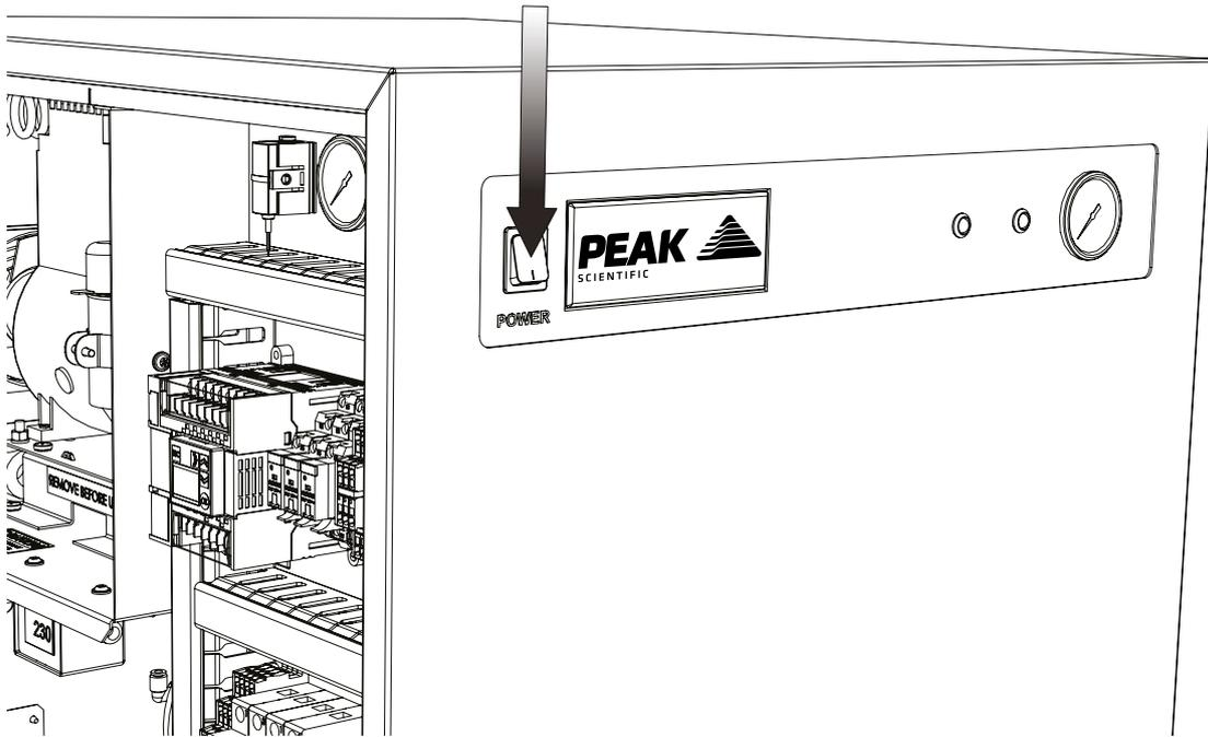
Switch the generator **OFF** using the switch on the front panel.
