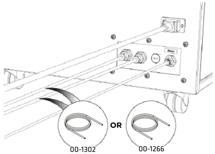
Attach the appropriate sized **Teflon tubing** to the fitting(s) attached to the **nitrogen port** and connect to the **gas inlet of your instrument**.
