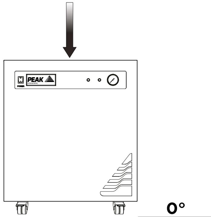
Unpack the generator from the shipping crate and position on a flat surface, in desired area.
