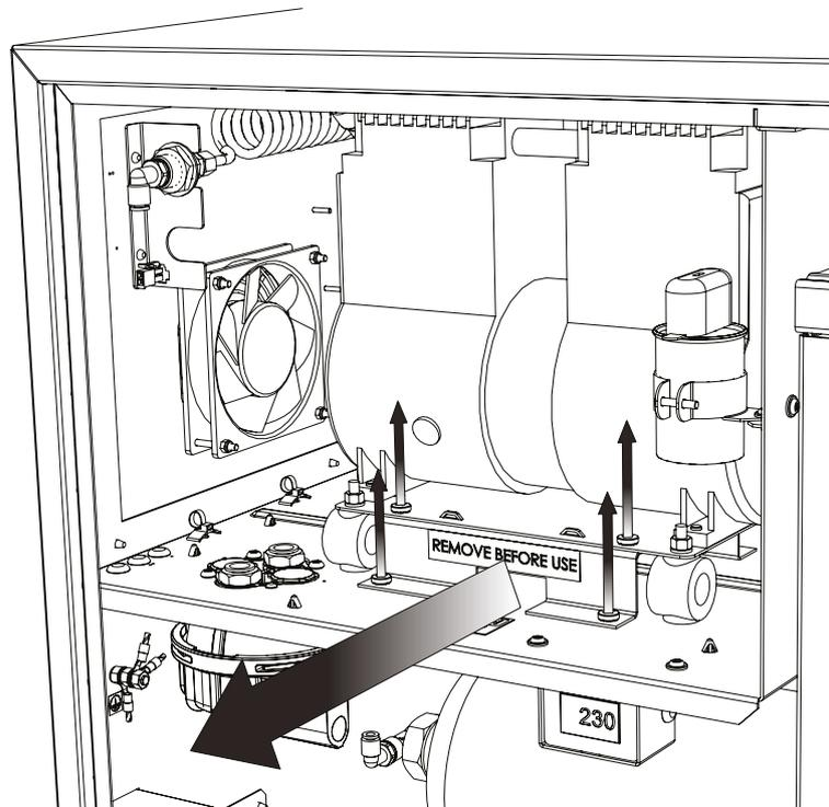
The **transit bracket** is located below the compressor and has a sticker on it stating 'Remove before use'. To remove the transit bracket, **remove the four screws** as indicated, then **slide the bracket out** from underneath the compressor. Please retain the bracket and screws for future transportation.
