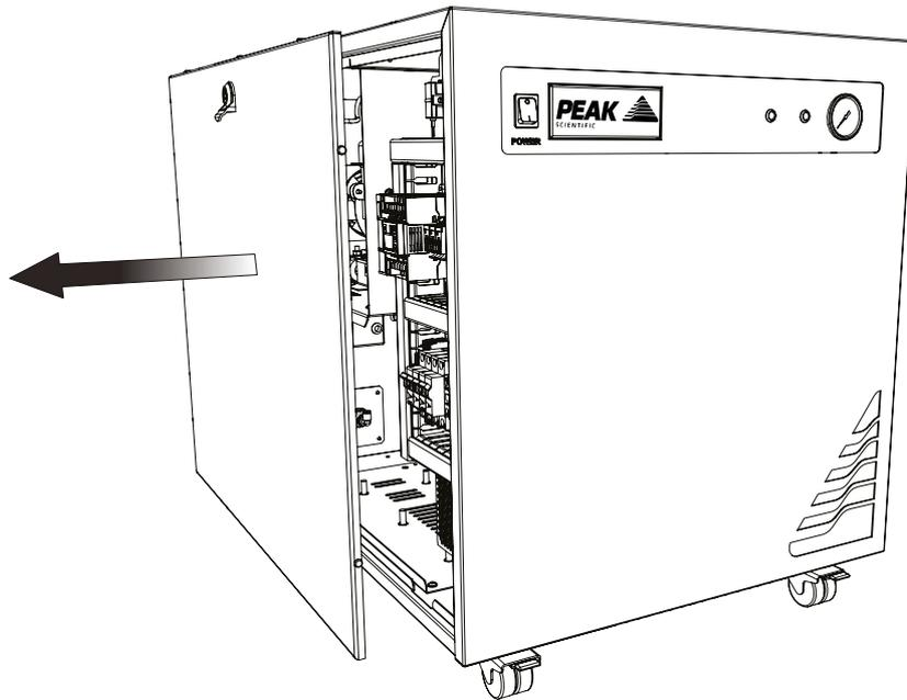
Once unlocked **remove the left hand side panel**, ensuring you **disconnect the earth lead** located in the lower middle of the panel.
