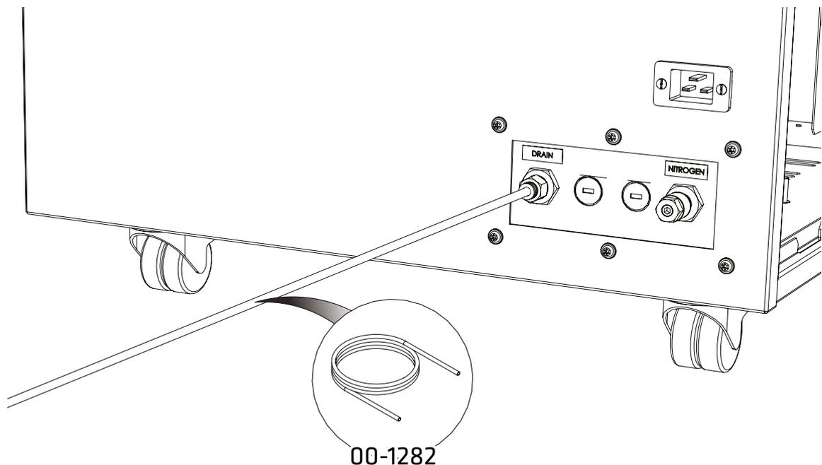
Connect the **6mm PE Tubing 00-1282** to the **1/4"- 6mm Push Fit Fitting 02-4600** connected to the **DRAIN port**. This will be either on the far left or far right of the panel.
