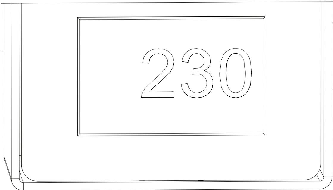
Check the Generators **internal voltmeter**. This will measure and display the mains voltage that is being supplied to the generator. Note the displayed voltage. If the voltage is 195V to 219V a transformer will be required. This can be ordered directly from Peak. **06-3200 Dual Tap Transformer 200-230V**
