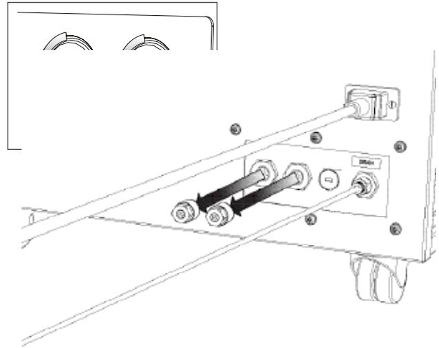
The purge is now complete. Once the pressure gauge(s) on the front of the generator read(s) 0, the **silencer fitting(s) can be removed** from the port(s).
