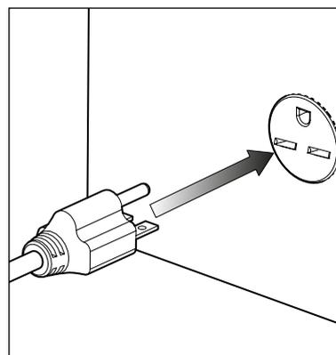
Plug the mains cable into the corresponding **100VAC 60Hz OR 230VAC 50/60Hz** single phase power supply.
